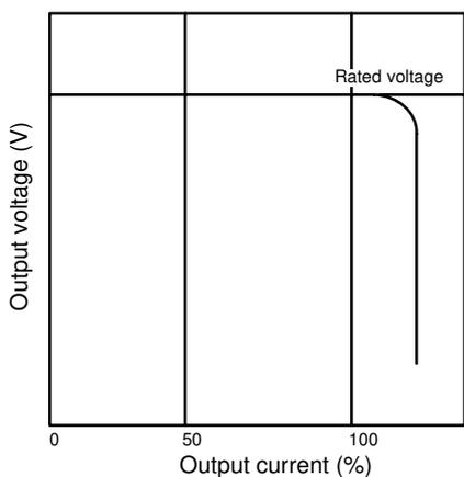
output. It operates at 105% min. of the rated current of +V output when -V output is producing the rated output, but this condition varies depending on -V output status. -V output has an independent short-circuit protection feature.
