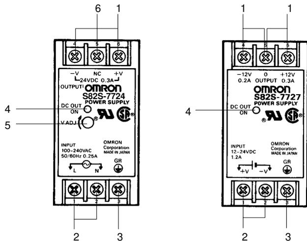
1. **DC Output Terminals:** Connect the load lines to these terminals.
