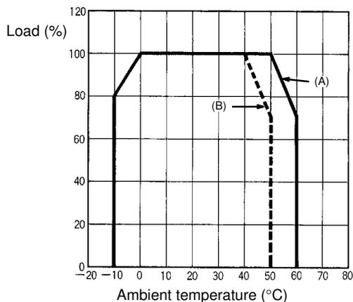
**Note:** The derating curve depends on the mounting direction of the Power Supply
