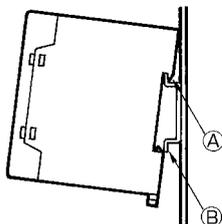
To dismount, pull down portion (C) with a screwdriver and pull out the power supply.
