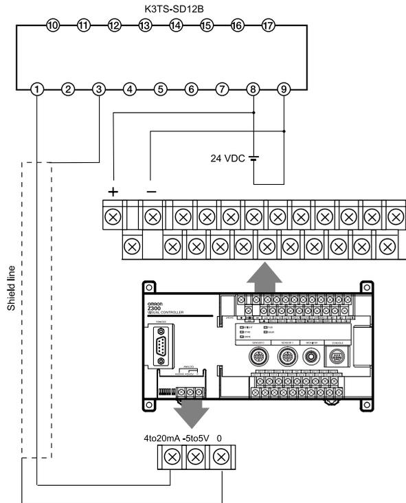
**Connecting to the Linear Sensor Controller (K3AS)**
