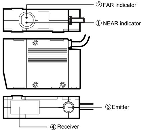
①,② If the distance between the front of the Sensor and the workpiece is the measurement range, these indicators turn ON or OFF according to the distance. If the workpiece is outside the measurement range or if the light density is insufficient, both indicators will flash.
