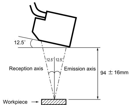
**CHECK** It is recommended that Sensor mounting is performed while monitoring the amount of received light in the menu item **Check position**.
