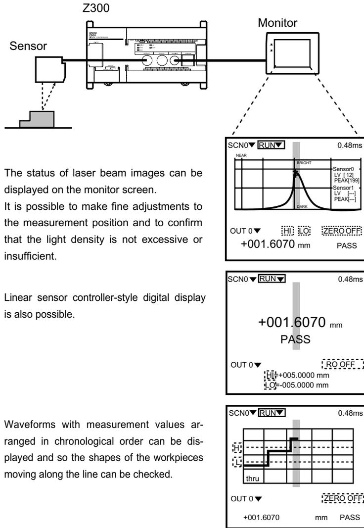
The status of laser beam images can be displayed on the monitor screen. It is possible to make fine adjustments to the measurement position and to confirm that the light density is not excessive or insufficient.
