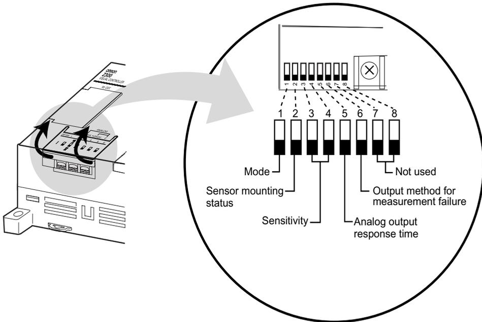
**Notice** Turn OFF the power supply before changing the DIP switch settings.
