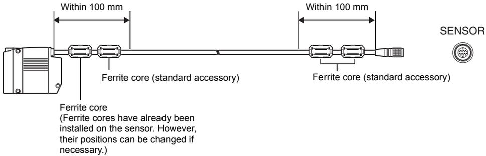
When using an extension cable, make sure that two ferrite cores are connected within 100 mm from the sensor and within 100 mm from the controller's connector, respectively.
