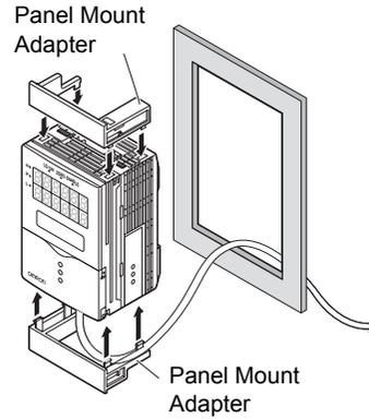
3. Install the long Mount Adapters on the two holes of the small Mount Adapter.
