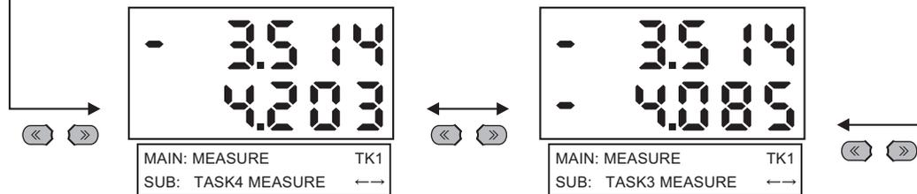
\*1) TKx on the LCD screen indicates that the measured value of the current TASKx is displayed in the main display. Switch TASK that is displayed in the main display by using the function keys.
