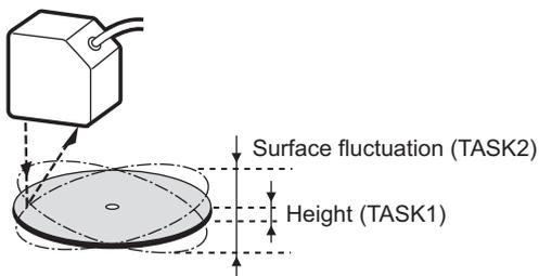
Measuring Multiple Items Simultaneously p.3-8
