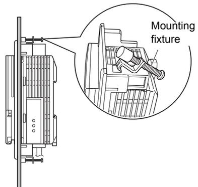
6. Make sure that the Sensor Controller is firmly fixed on the panel.
