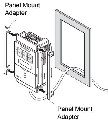
4. Install the Sensor Controller with Panel Mount Adapters attached onto the panel from the front.
