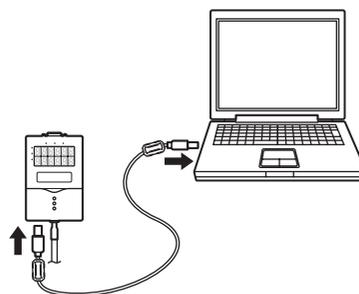
“Detected new hardware” will be displayed on the Windows tool bar, and the [New Hardware Detection Wizard] dialog box will appear.
