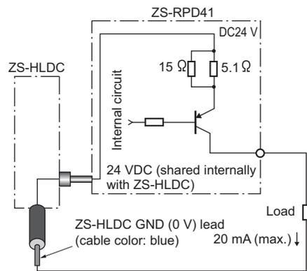
**Assignment of Terminal Block Output**
