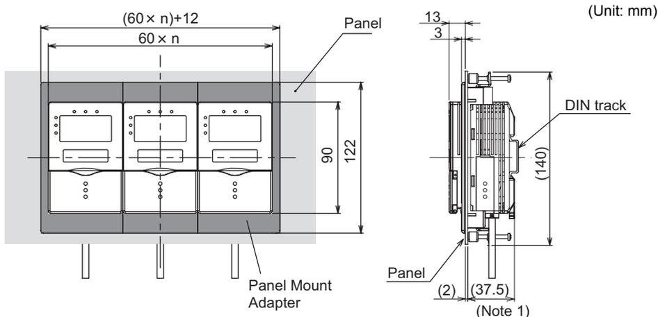
Note 1: Dimensions are shown for a panel thickness of 2.0 mm.
