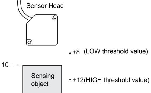
Example 3: Using zero reset to measure steps in sensing object (zero reset at each measurement)
