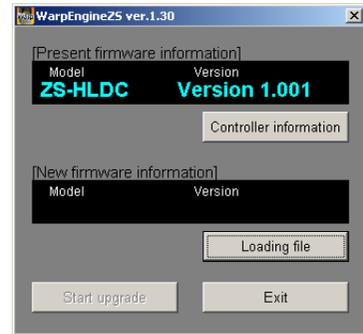
When the startup of Warp Engine ZS fails, the following screen is displayed after a message appears. Go to “Set the connection port”.
