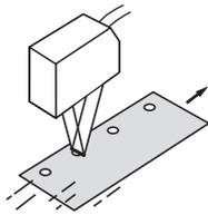
Abnormal values such as spiking that occur when the shape of the workpiece suddenly changes during measurement.
