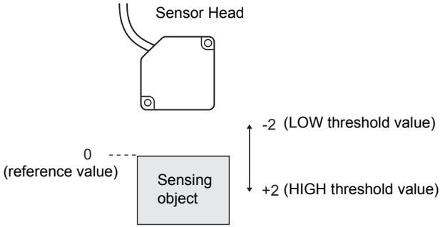
Example 2: Using the height of sensing object as the measured value with an offset set to 10
