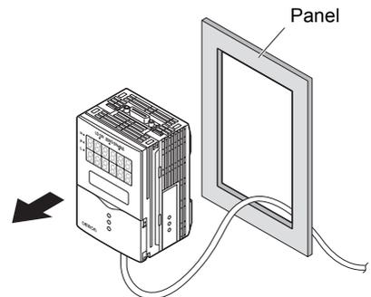
2. Install the small Mount Adapters on the four holes of the Sensor Controller.
