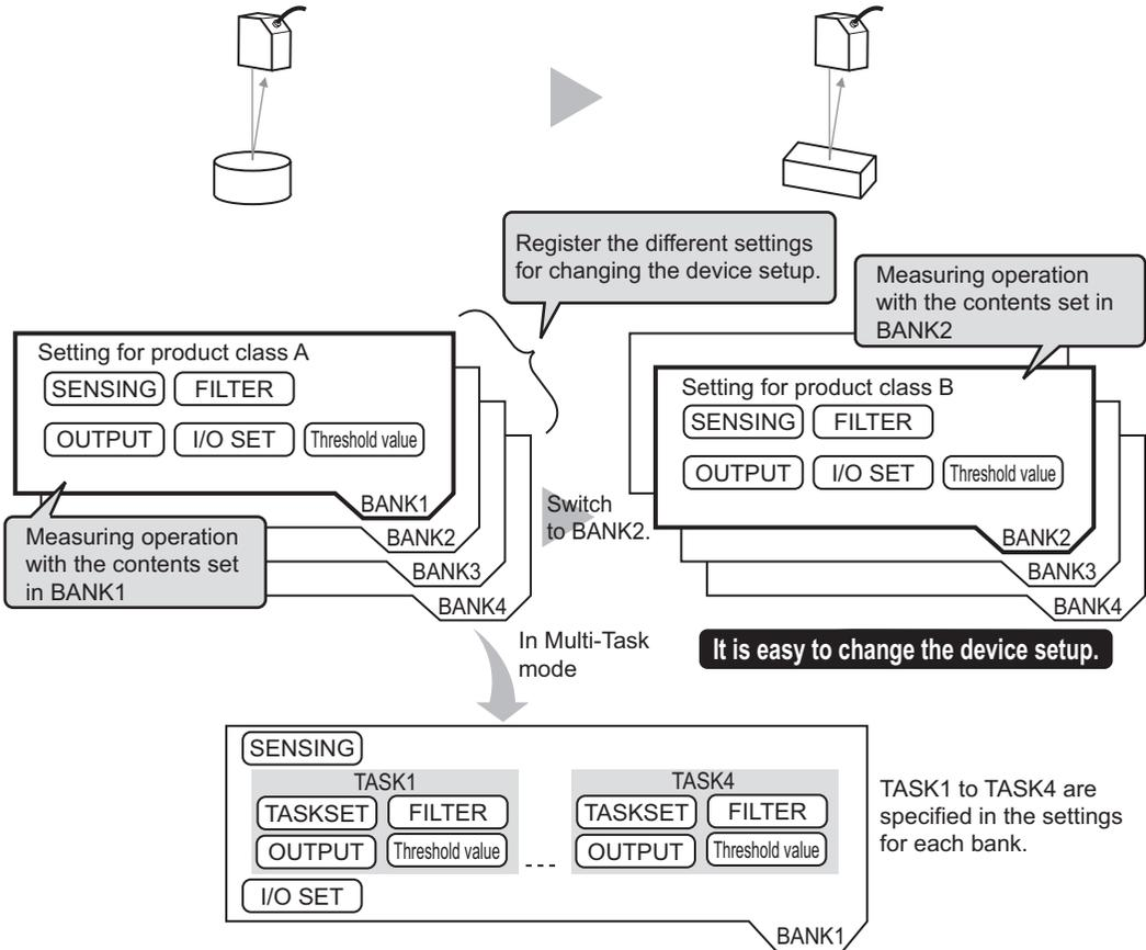
If only the "threshold value" is different in the settings for a bank, by changing the mode of the bank, you can increase the number of banks from 4 to 32.
