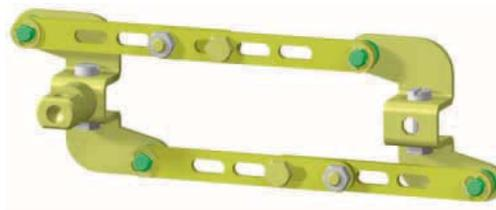
Mechanical interlocks for parallel switching are for simultaneous switching of two circuit breakers. Parallel switching can be used between two 3VT1 circuit breakers. Each circuit breaker must be furnished with a manual operating unit and at least one with a knob (see page 2/25). In order to use parallel switching, it is absolutely necessary to comply with the dimensions shown in the figure and given in the table.
