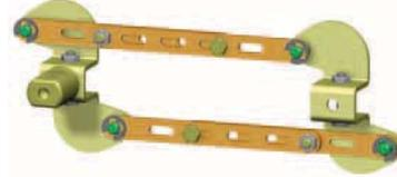
Provides for simultaneous switching of two circuit breakers/switch disconnectors. Parallel switching can be used between two 3VT2 circuit breakers or between 3VT2 and 3VT3 circuit breakers. Each circuit breaker must be equipped with a rotary operating mechanism and at least one with a knob.
