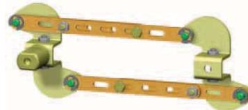
Provides for simultaneous switching of two circuit breakers/switch-disconnectors. Parallel switching can be used between two 3VT3<sup>1)</sup> circuit breakers or between 3VT3 and 3VT2 circuit breakers. Each circuit breaker must be equipped with a manual operating mechanism and at least one with a knob, see page 4/48. In order to use parallel switching it is absolutely necessary to comply with the dimensions shown in the figure and table.
