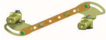
Provides mechanical interlocking of two circuit breakers/switch disconnectors so that they cannot both be tripped simultaneously, but only one of them at the same time. Both circuit breakers may be turned off simultaneously. Interlocking can be used between two 3VT2 circuit breakers or between one 3VT2 and one 3VT3 circuit breaker. Both circuit breakers must be furnished with a rotary operating mechanism (at least one with a rotary operating mechanism and knob).
