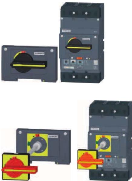
The rotary operating mechanism makes possible to govern the circuit breaker by pivoting lever, e.g. to switch machines on and off. Modular conception of drives makes possible simple mounting on the switching unit (also additionally) after the accessory compartment cover is removed. A fixed motor is possible to seal. The drive and its accessories is ordered separately according to your choice (see page 4/6).
