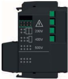
The particular rated operating voltage of the shunt release is set up by jumpers located on the right hand side in the release. It is always set to the maximum value by default.
