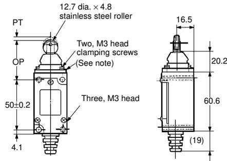
**Note:** The head can be mounted in either of the two directions. Dimensions not shown are the same as HL-5000.
