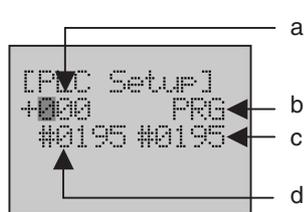
5. Press the **OK** button to enter the PLC Setup Screen
