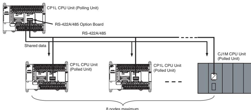
**1:1 Connections between CP1L/CJ1M CPU Units**
