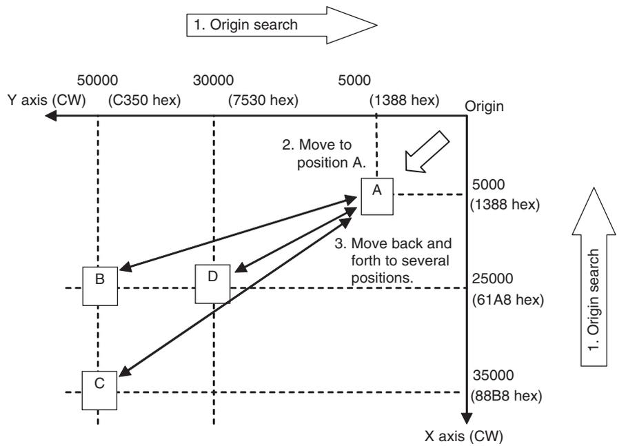
**Note** The X and Y axes are moved independently, i.e., interpolation is not performed.
