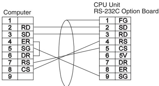
Connecting a Host Computer with NT-AL001 Converting Link Adapters
