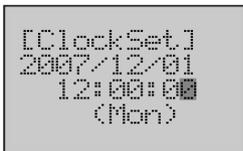
6. Use the **Forward** button to move the column cursor to the position of PLC time. Use the **Down** or **Up** button to change the time to **12:00:00**.
