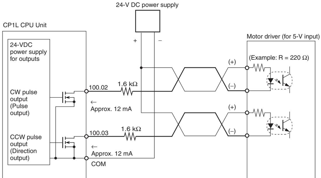
In this example, a 5-V input motor driver is used with a 24-VDC power supply. Be careful to ensure that the Position Control Unit output current does not damage the input circuit at the motor driver and yet is sufficient to turn it ON. Take into account the power derating for the 1.6-kΩ resistance.
