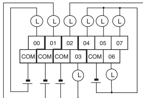
**CP1W-20EDT1/CP1A-20EDT1 (Sourcing Transistor Outputs)**
