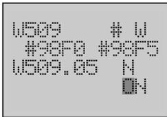
16. Use the **Forward** button to move the column cursor to the bit state position. The present state is ON. The state ON or OFF is according to PLC.
