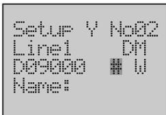
13. Use the **Forward** button to move the column cursor to the display format position.
