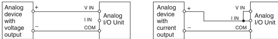
**Wiring for Analog Outputs**
