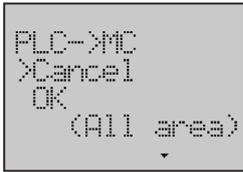
6. Press the **OK** button to enter the "PLC->MC" Operation Screen.
