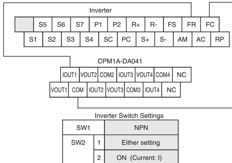
■ Inverter Connections to Motor
