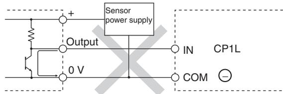
**Precautions when Connecting a Two-wire DC Sensor**
