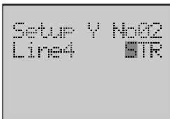
7. Use the **Forward** button to move the column cursor to the display type position.
