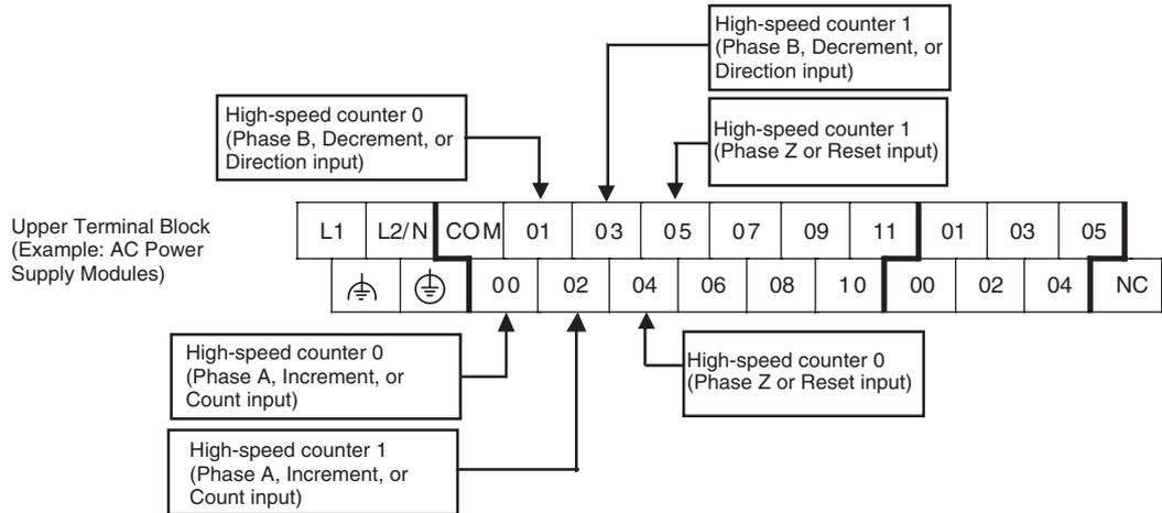
**Input Terminal Arrangement for CPU Units with 40 I/O Points**
