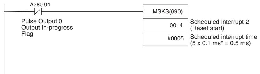
\* Select 0.1 ms for the setting units in the PLC Setup.
