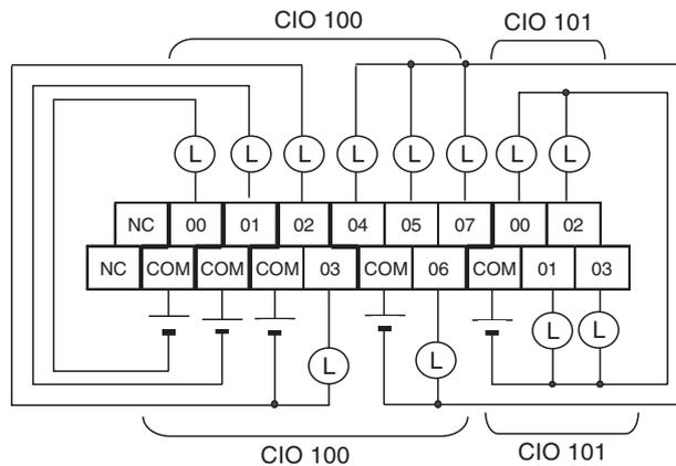
**3-5-4 I/O Wiring for CPU Units with 20 I/O Points**
