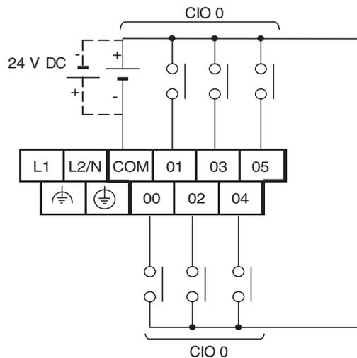
**Output Wiring (Lower Terminal Block, not Removable)**
