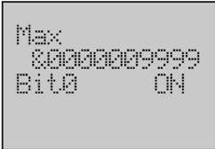
1. Press the **Forward + OK** button simultaneously to enter the Data Change Screen.
