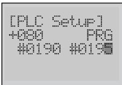
7. Use the **Forward** button to move the column cursor to the value of PLC Setup.
