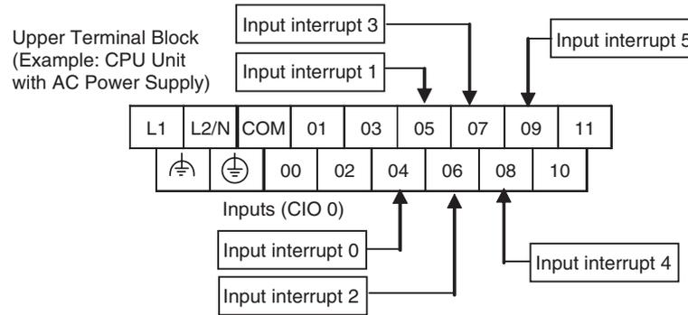
**Input Terminal Block of CPU Units with 30 I/O Points**
