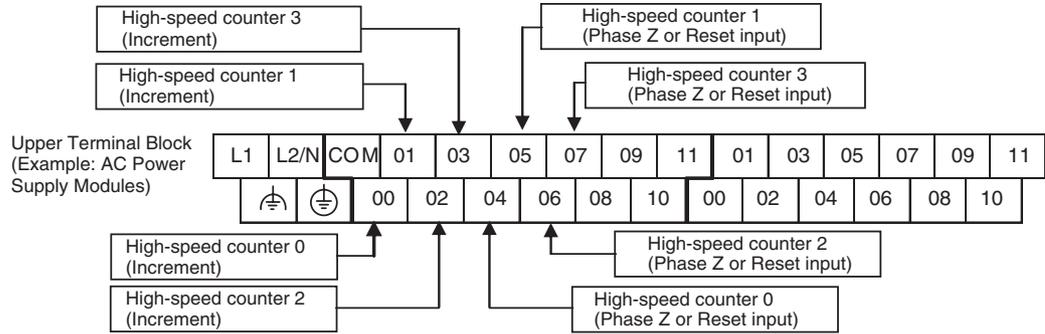
**Input Terminal Arrangement for CPU Units with 60 I/O Points**
