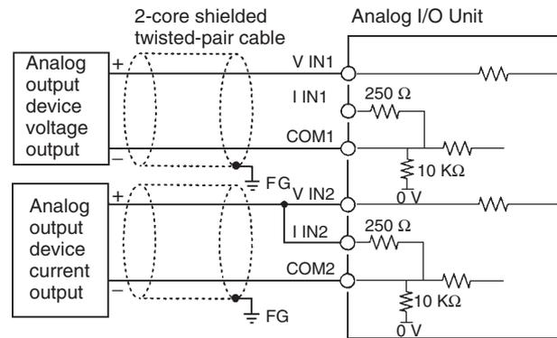
**Analog I/O Wiring Example**
