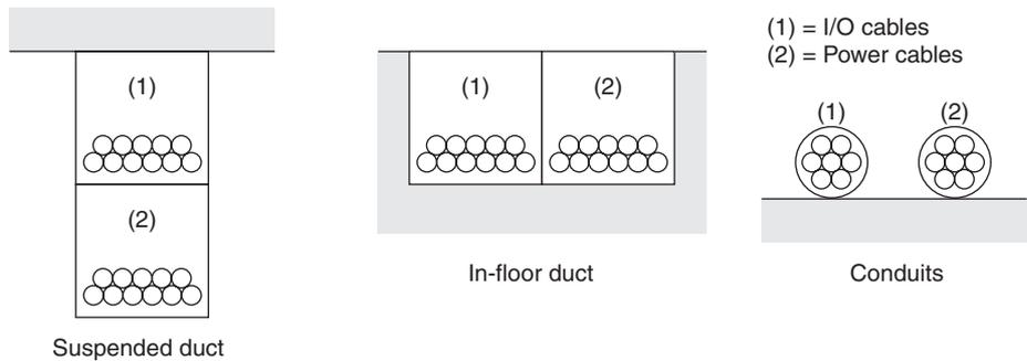
If the I/O wiring and power wiring must be routed in the same duct, use shielded cables and connect the shields to the GR terminal to reduce noise.
