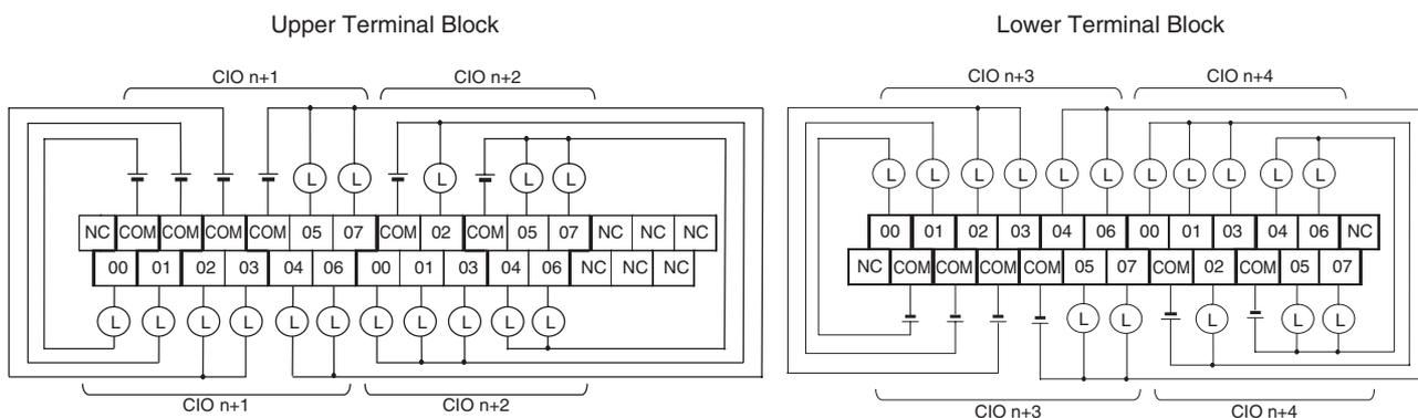
**Output Wiring CP1W-32ET1 (Sourcing Transistor Outputs)**
