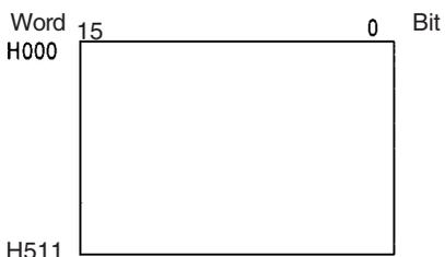
**Note** H512 to H1535 are used as a Function Block Holding Area. These words can be used only for function block instances (internally allocated variable area). These words cannot be specified as instruction operands in the user program.
