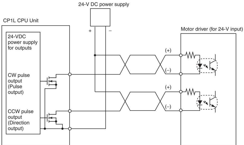
**Using a 5-VDC Photocoupler Input Motor Driver (CP1L-□□□DT-D)**
