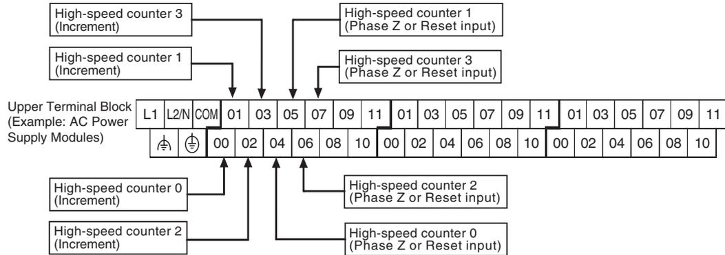
**Input Function Settings in the PLC Setup**
