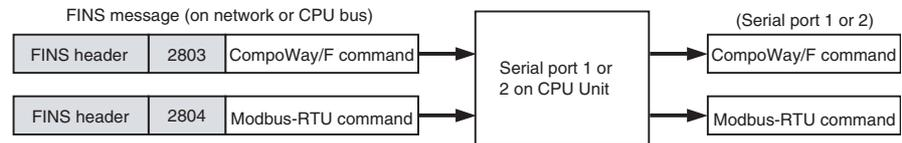
The serial gateway functionality is enabled when serial port 1 or 2 is set to the Serial Gateway Mode.
