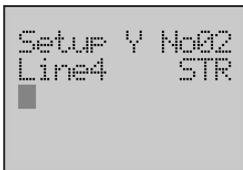
8. Use the **Forward** button to move the column cursor to the position of String Name.
