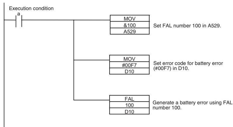
**Note** Use the same methods as for actual system errors to clear the simulated system errors. Refer to the *11-2 Troubleshooting* for details. All system errors simulated with FAL(006) and FALS(007) can be cleared by cycling the power supply.
