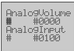
4. Press the **OK** button to enter the Monitor Screen of analog setting.
