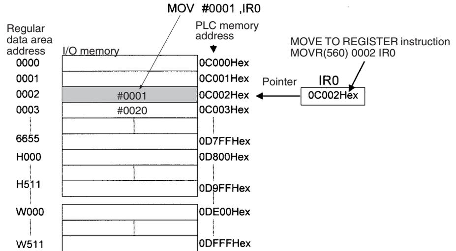
**Note** The PLC memory addresses are listed in the diagram above, but it isn't necessary to know the PLC memory addresses when using Index Registers.
