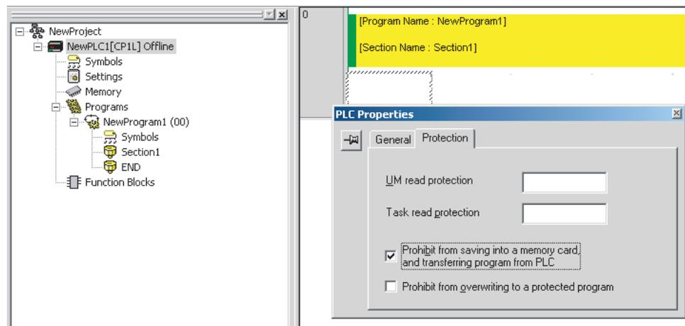
2. Go online and then either select **PLC - Transfer - To PLC** to transfer the program or select **PLC - Protection - Set Password** and click the **OK** button.
