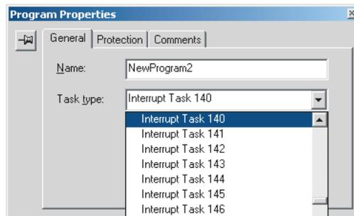
If you click the **X** Button in the upper-right corner of the window, you can create the program that will be executed as interrupt task 140. The programs allocated to each task are independent and an END(001) instruction must be input at the end of each program.
