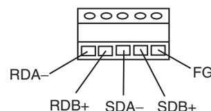
Tighten the terminal block screws to a torque of 0.28 N·m (2.5 Lb In.).
