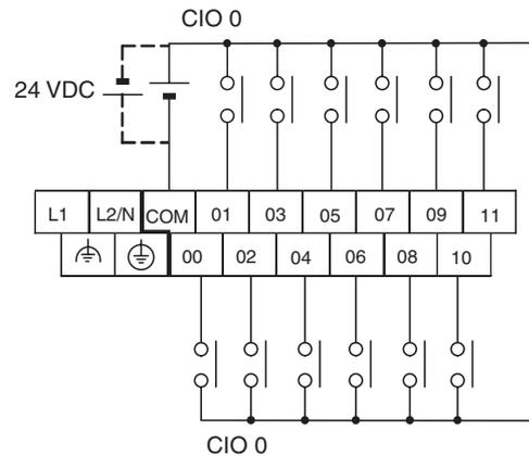
**Output Wiring (Lower Terminal Block, not Removable)**
