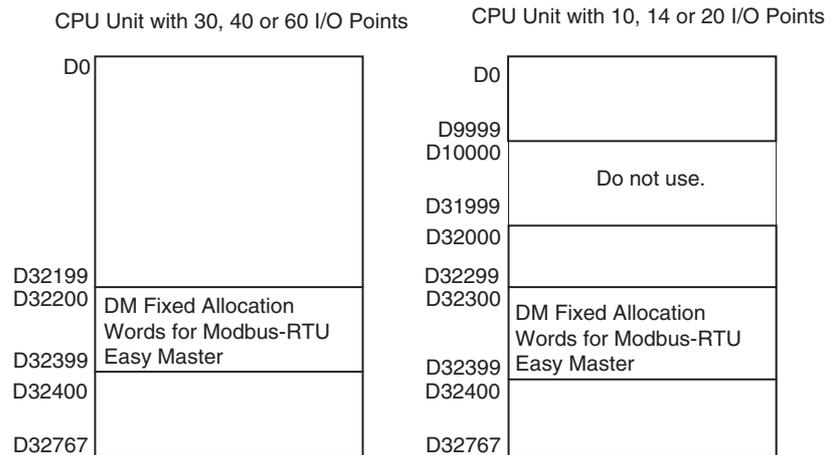
This data area is used for general data storage and manipulation and is accessible only by word.
