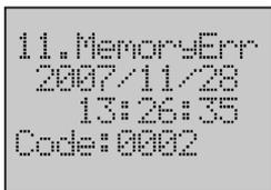
6. If there is more than one error, press the **Down** button to scroll the screen and display the details of the next error.
