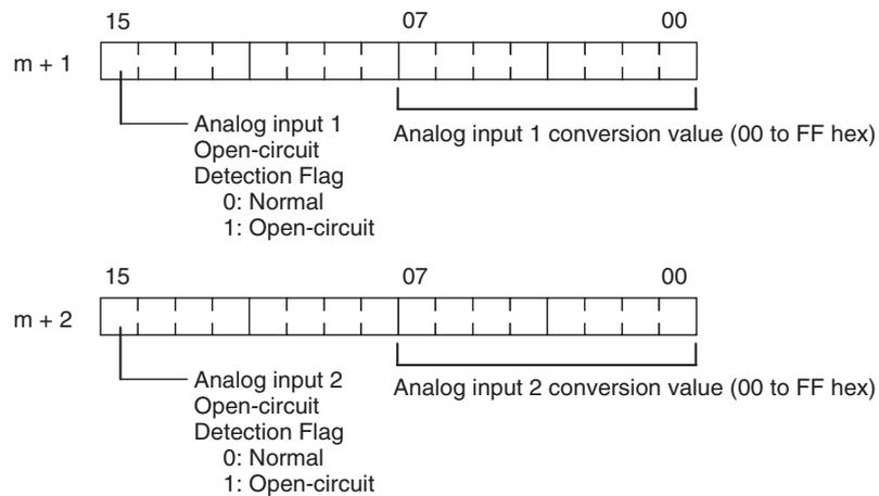
**Note** The Open-circuit Detection Flag is turned ON if the input signal range is set to 1 to 5 V or 4 to 20 mA and the input signal falls below 1 V or 4 mA. (Open circuits are not detected when the input signal range is set to 0 to 10 V.)
