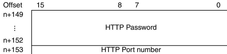
If the password for accessing the Ethernet Option Board's Web page is forgotten, find out it in this area. It is written in ASCII format.
