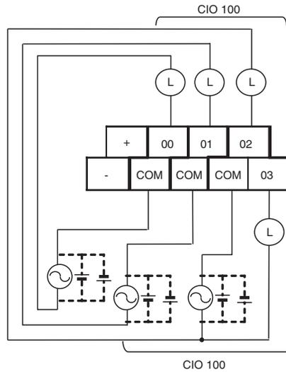
AC-power-supply models have a 24-VDC output terminals (+/-) on the lower terminal block. They can be used as a DC power supply for the input circuit.
