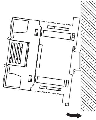
3. Press in all of the DIN Track mounting pins to securely lock the Units in place.
