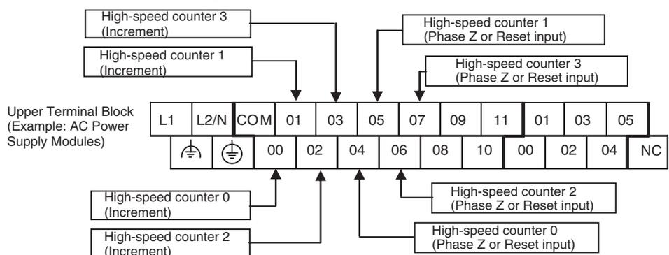
**Input Terminal Arrangement for CPU Units with 40 I/O Points**
