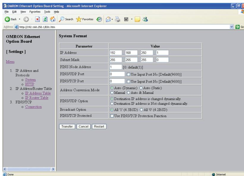
5. Make the required settings (i.e., the IP address in this example).
