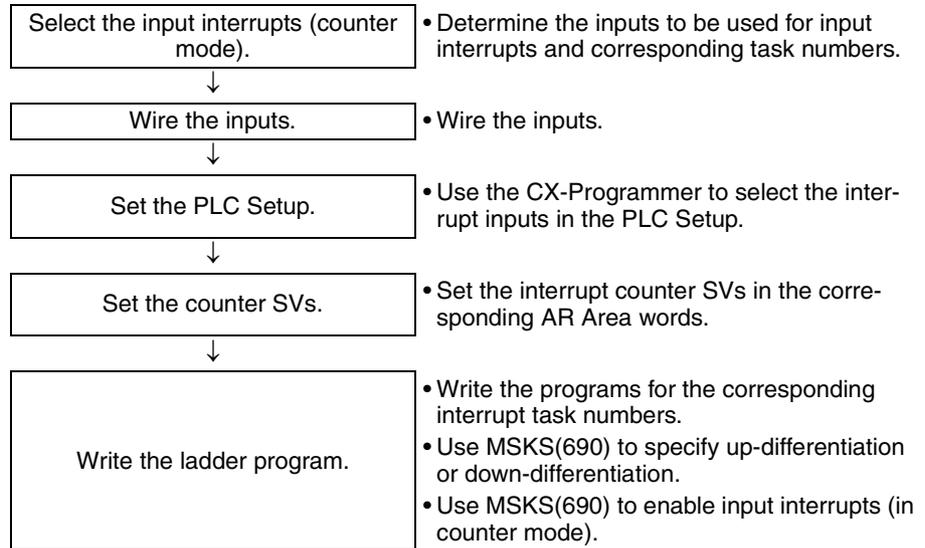
**Note** The input interrupt (counter mode) function is one of the input interrupt functions and executes an interrupt based on the pulse count. If the input pulse frequency is too high, interrupts will occur too frequently and prevent normal cyclic task processing. In this case, cycle time too long errors may occur or the pulse input may not be read.
