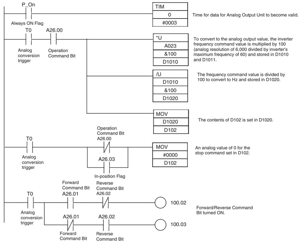
In this example, the results of \*U and /U are 1, so the value in A23 is moved directly to D102 with MOV.
