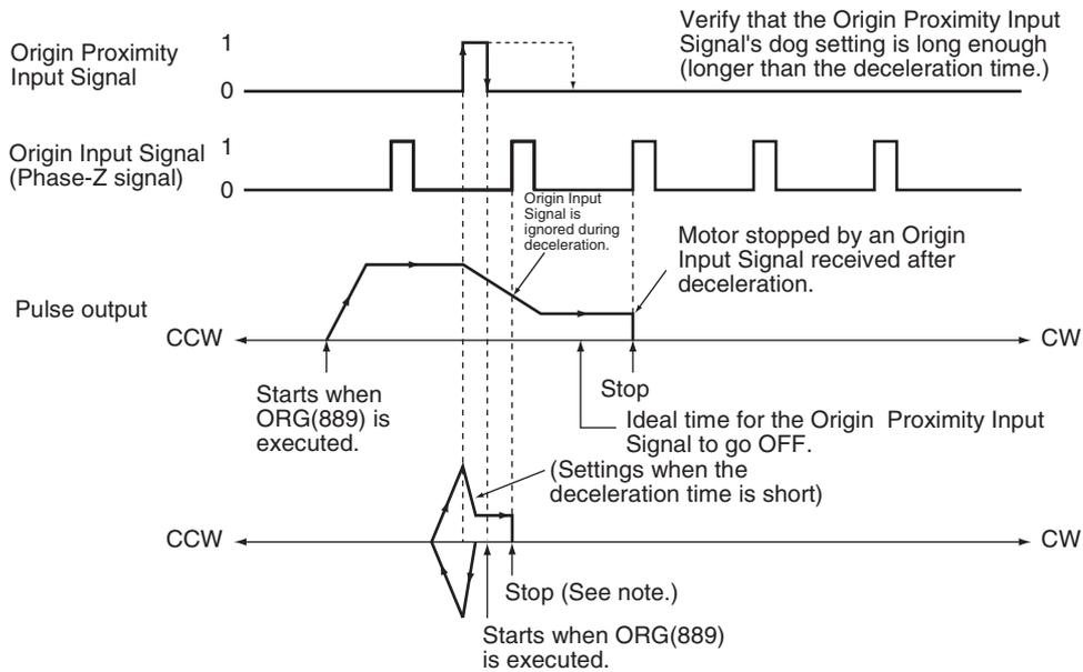
**Note:** The Origin Input Signal can be detected immediately after the Origin Proximity Input Signal goes from ON to OFF if the deceleration time is short, e.g., starting from within the Origin Proximity Input Signal.
