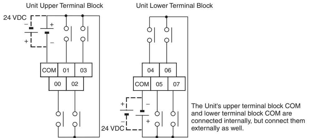
**8-point Output Units (CP1W/CPM1A-8E□) (Terminal Block is not Removable)**
