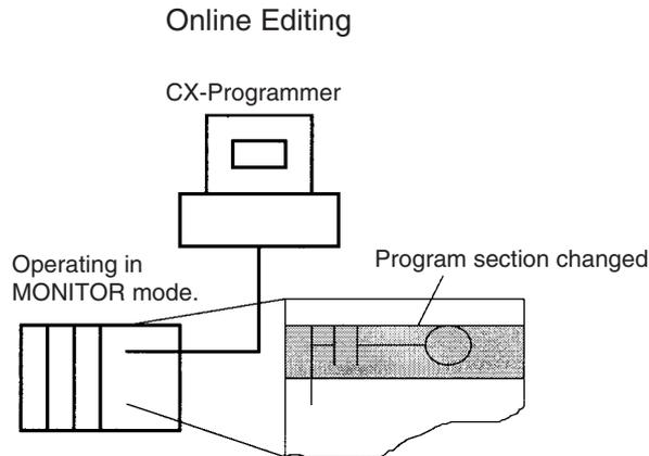
The cycle time will be increased by from one to several cycle times if the program in the CPU Unit is edited online in MONITOR mode. The cycle time will also be increased to back up data in the flash memory after online editing. The BKUP indicator will be lit during this period and the progress of the backup will be displayed on the CX-Programmer. The increases per cycle are listed in the following table.
