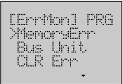
5. Press the **OK** button to enter the Error Monitor Screen.
