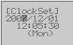
5. Press the **OK** button to enter the Clock Setup Screen. The present date, time and week of the CPU Unit will be displayed.
