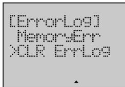
7. Press the **ESC** button to return to the Error History Screen. Press the **Down** button to select **CLR ErrLog** which is always below the last error.
