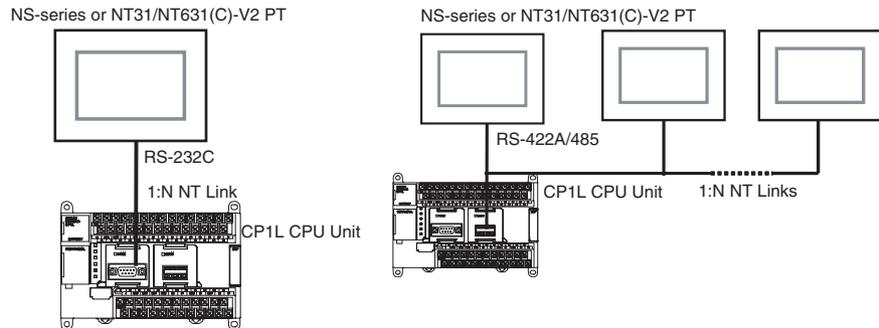
**Note** Communications are not possible using the 1:1-mode NT Link protocol.
