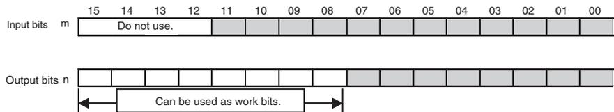
One input word (12 bits) and one output word (8 bits) are allocated for a 20-point Expansion I/O Unit.
