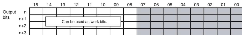
Four words (32 bits) are allocated to a 32-output Expansion Output Unit. No input words are allocated. Output bits 08 to 15 can be used as work bits.
