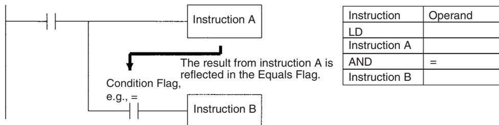
Since the Condition Flags are shared by all of the instructions, program operation can be changed from its expected course by interruption of a single task. Be sure to consider the effects of interrupts when writing the program. Refer to *SECTION 2 Programming of CS/CJ Series Programming Manual (W394)* for more details.
