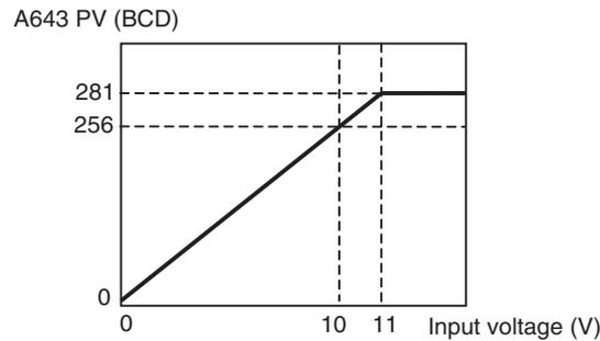
The maximum input voltage is 11 VDC. Do not apply a voltage greater than that.
