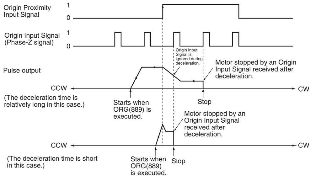
**Operating Mode 2 (with Error Counter Reset Output, with Positioning Completed Input)**
