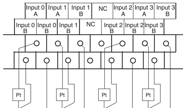
Temperature input 0    Temperature input 1    Temperature input 2    Temperature input 3
