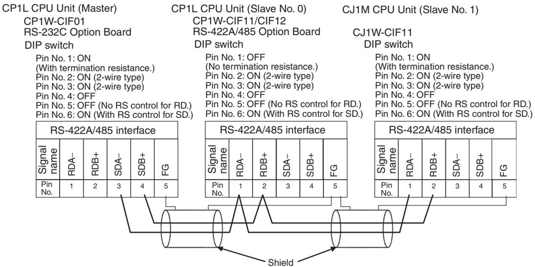
**Connections in Loopback Test**
