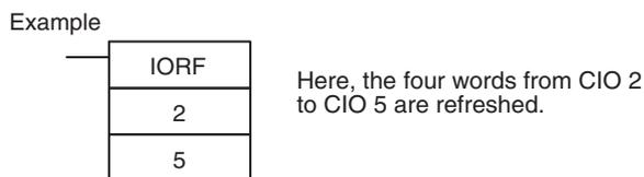
If high-speed response is required from input to output, execute IORF(097) before and after the relevant instructions.
