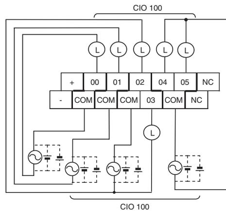
AC-power-supply models have a 24-VDC output terminals (+/-) on the lower terminal block. They can be used as a DC power supply for the input circuit.
