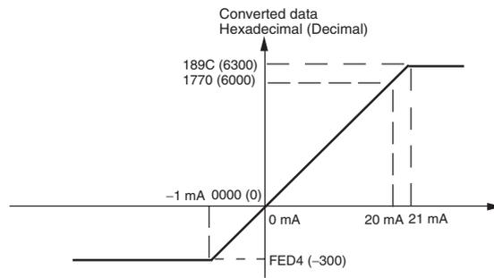
Current in the 0 to 20 mA range corresponds to hexadecimal values 0000 to 1770 (0 to 6,000). The range of data that can be converted is FED4 to 189C hex (-300 to 6,300). A negative current is expressed as two's complement.
