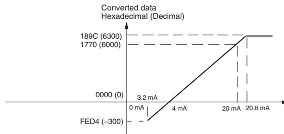
Current in the 4 to 20 mA range corresponds to hexadecimal values 0000 to 1770 (0 to 6,000). The range of data that can be converted is FED4 to 189C hex (-300 to 6,300). Current in the range of 3.2 to 4 mA is expressed as two's complement.
