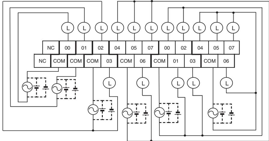
**CP1W-40EDT/CPM1A-40EDT (Sinking Transistor Outputs)**
