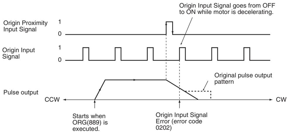
**Operating Mode 1 (with Error Counter Reset Output, without Positioning Completed Input)**
