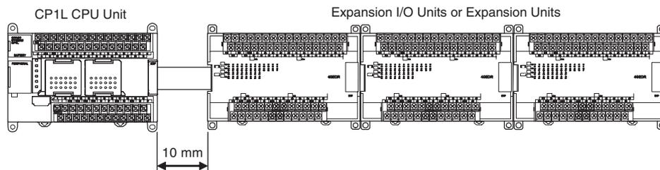
If sufficient space cannot be provided between the CPU Unit and the first Expansion Unit or Expansion I/O Unit, use the PLC in an ambient temperature of 0 to 50°C.
