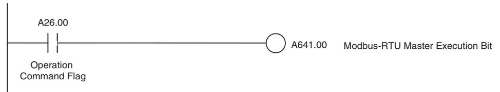
Add the above instructions to the end of the program as a starting condition for the ladder programming example. For error processing, refer to the ladder program in 6-3-3 Modbus-RTU Easy Master Function and to the inverter's manual.
