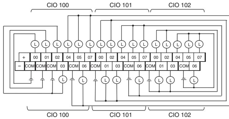
AC-power-supply models have a 24-VDC output terminals (+/-) on the lower terminal block. They can be used as a DC power supply for the input circuit.
