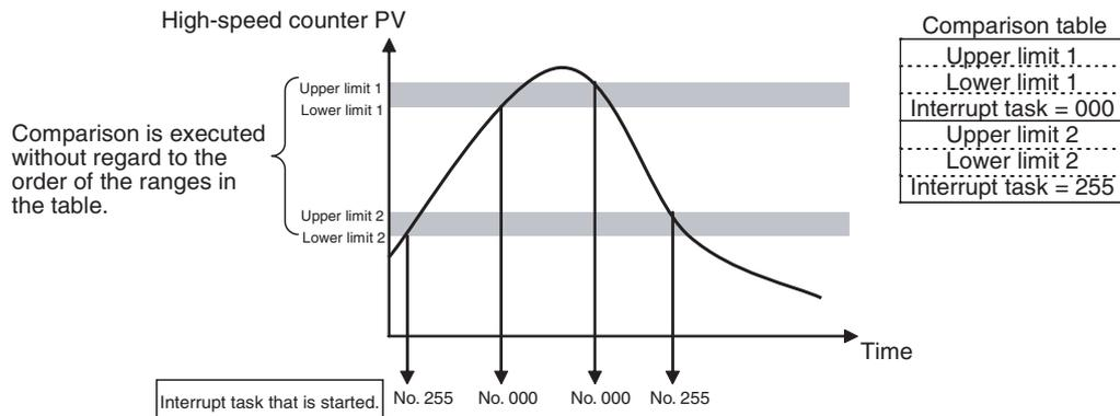
**Note** The range comparison table can be used without starting an interrupt task when the comparison condition is met. The range comparison function can be useful when you just want to know whether or not the high-speed counter PV is within a particular range. Use the Range Comparison Condition Met Flags to determine whether the high-speed counter PV is within a registered range.
