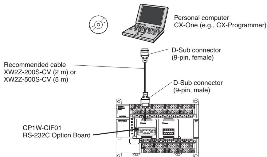
Connect the CX-Programmer to the RS-232C port of the CP1W-CIF01 Option Board by XW2Z-200S-CV/500S-CV RS-232C cable.
