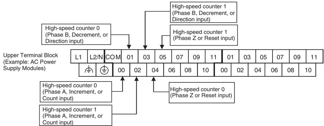
**Input Terminal Arrangement for CPU Units with 60 I/O Points**
