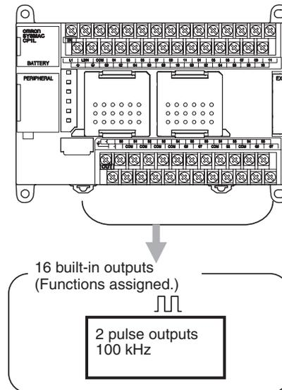
**Note** The instruction used to control each output point determines whether it is used as a normal output, pulse output, or PWM output.
