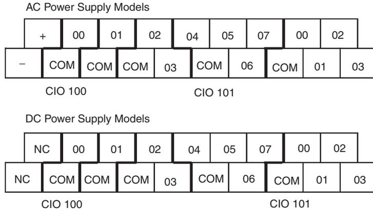
**Setting Output Functions Using Instructions and PLC Setup**
