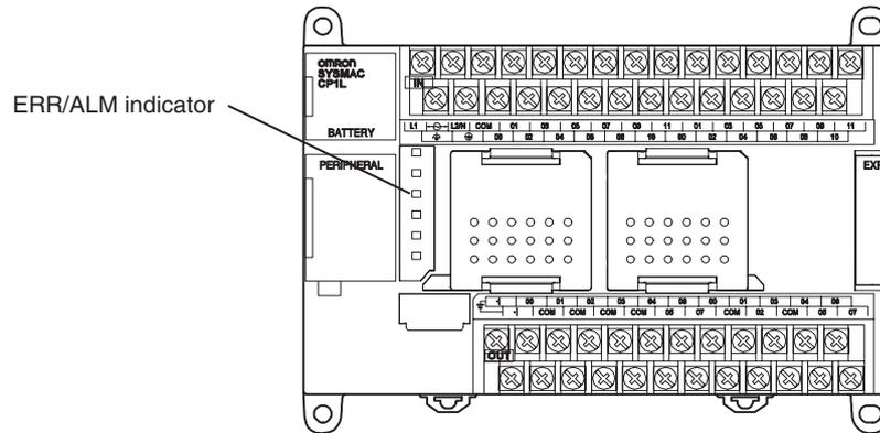
When the ERR/ALM indicator flashes, connect the CX-Programmer to the peripheral port and read the error messages. If a low battery message appears on the CX-Programmer (see note 1) and the Battery Error Flag (A402.04) is ON (see note 1), first check whether the battery is properly connected to the CPU Unit. If the battery is properly connected, replace the battery as soon as possible.
