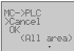
4. Press the **OK** button to enter the "MC->PLC" Operation Screen.
