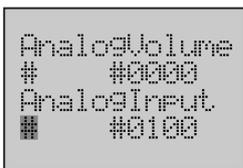
5. Use the **Forward** button to move the column cursor to the display format position on line 4.
