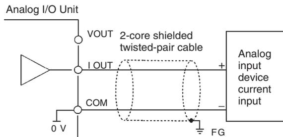
**Analog I/O Wiring Example**
