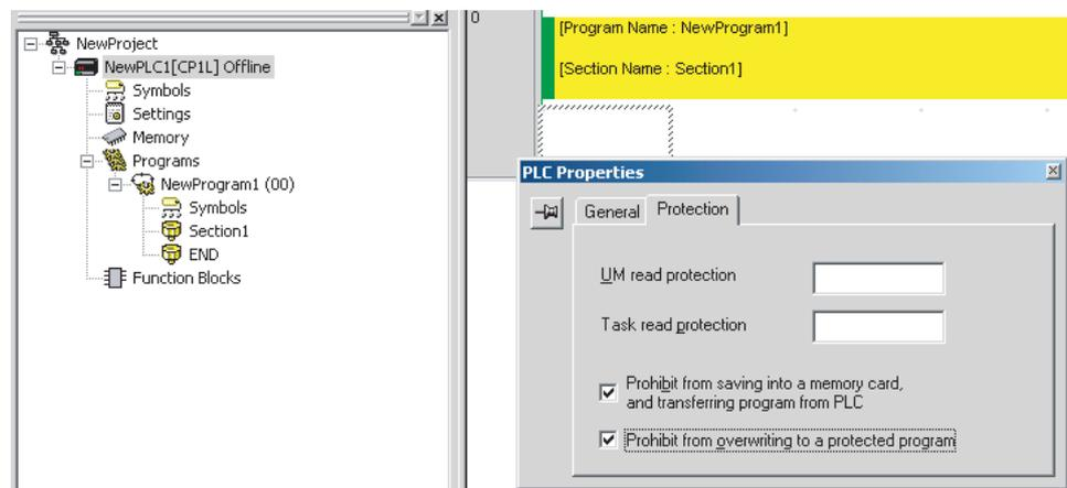
3. Either select **PLC - Transfer - To PLC** to transfer the program or select **PLC - Protection - Set Password** and click the **OK** button.
