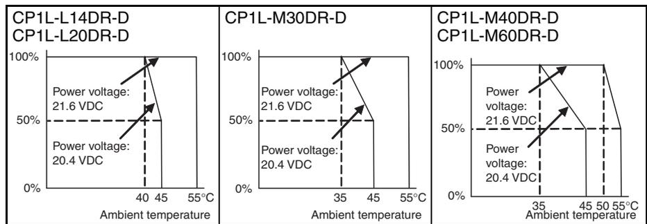
**Note** The above restrictions, apply to the relay output load current from the CPU Unit even if Expansion I/O Units are not connected.
