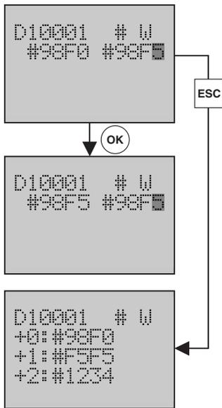
3. Use the **Forward** button to move the column cursor to the data of I/O memory. Use the **Down** or **Up** button to change the value of each digit.
