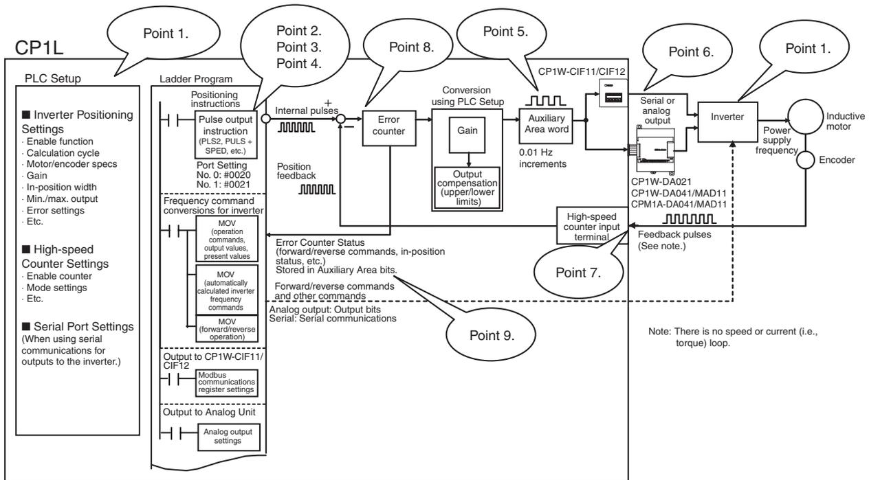
1. To use inverter positioning, the motor and encoder specifications, feedback gain, and other parameters must be set in the PLC Setup. The high-speed counter and inverter must also be set.
