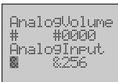
6. Press the **Down** or **Up** button to change the display format to **&**.
