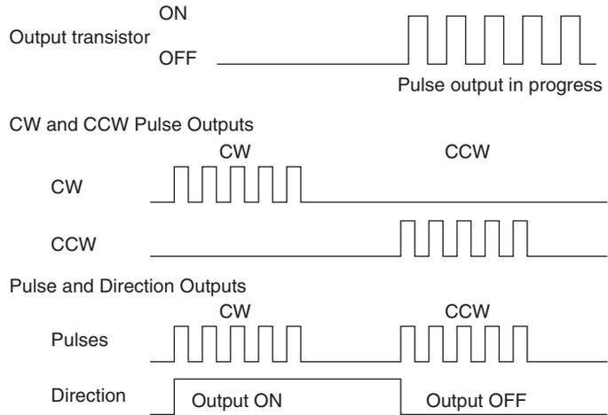
**CW/CCW Pulse Output and Pulse Plus Direction Output**
