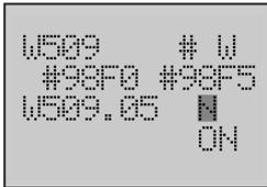
15. Use the **Forward** button to move the column cursor to the bit flag position. The present setting is the default setting. Select the bit flag in the following table.
