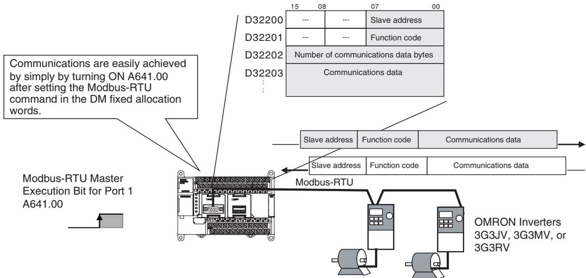
**DM Fixed Allocation Words for the Modbus-RTU Easy Master**
