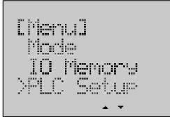
2. Press the **Down** button to select **PLC Setup**.
