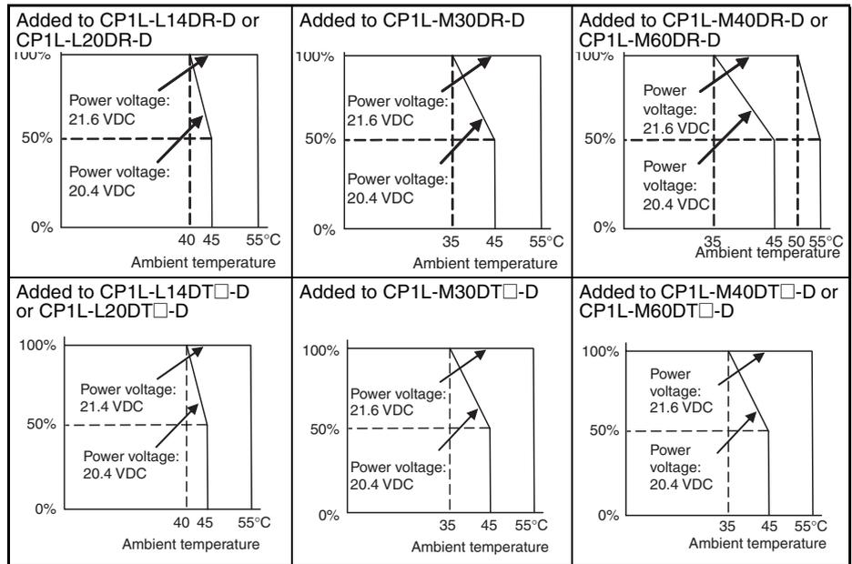
Transistor Outputs (Sinking or Sourcing)
