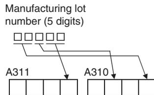
X, Y, and Z in the lot number are converted to 10, 11, and 12, respectively, in A310 and A311. Some examples are given below.
