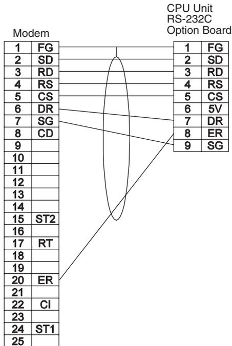
1:N Connections Using RS-232C Ports
