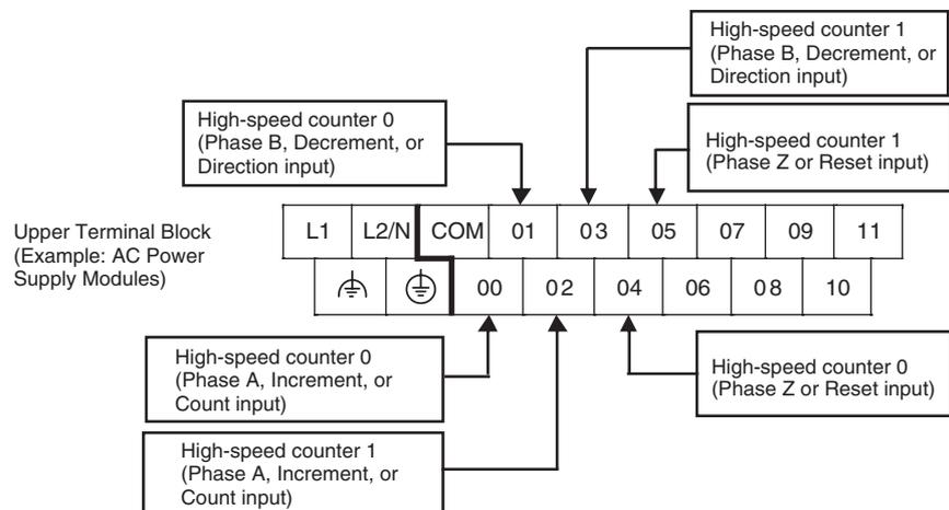
**Input Terminal Arrangement for CPU Units with 30 I/O Points**
