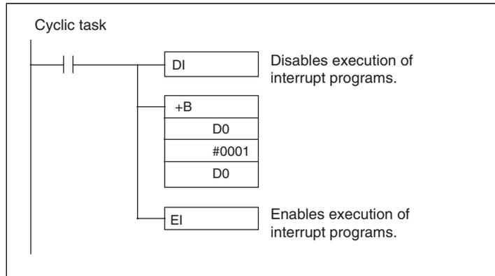
b. The following example shows duplicate processing by an interrupt task, which interrupts processing while BSET is writing to a block of words and yields an incorrect comparison result.
