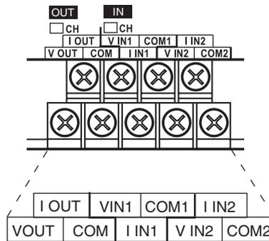
**Note** When using current inputs, short terminal V IN1 with I IN1 and terminal V IN2 with I IN2.
