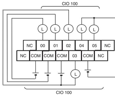
**3-5-6 I/O Wiring for CPU Units with 10 I/O Points**
