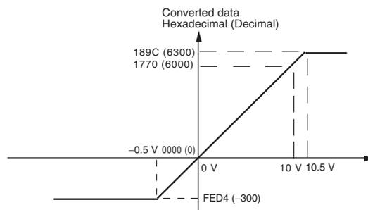
Voltage in the 0 to 10 V range corresponds to hexadecimal values 0000 to 1770 (0 to 6,000). The range of data that can be converted is FED4 to 189C hex (-300 to 6,300). A negative voltage is expressed as two's complement.
