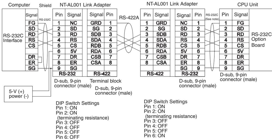
**Note** We recommend using the following NT-AL001 Link Adapter Connecting Cables to connect to NT-AL001 Link Adapters.
