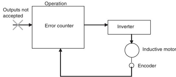
**Referencing the Automatically Calculated Inverter Frequency Command Value**
