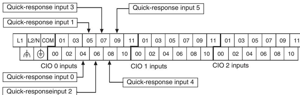
**Setting the Input Functions in the PLC Setup**
