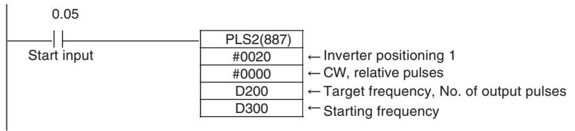
**Note** The pulse output method (CCW/CW or pulse + direction) setting and direction setting are not used.
