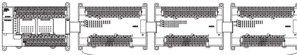
A maximum of three CP-series Expansion I/O Units or Expansion Units can be added.
