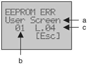
1. A flashing error screen will be displayed when an error occurs. The following table shows the display items.
