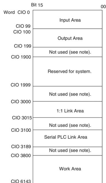
**Note** The parts of the CIO Area that are labelled “not used” may be used in programming as work bits. In the future, however, unused CIO Area bits may be used when expanding functions. Always use Work Area bits first.
