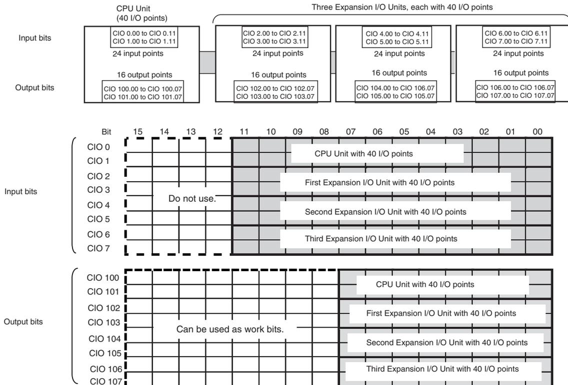
**Example 2: Connecting Expansion I/O Units with Only Inputs or Only Outputs**
