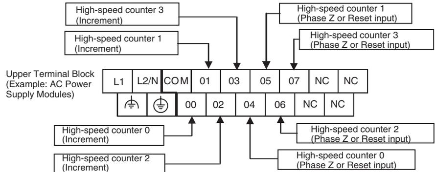
Input Terminal Arrangement for CPU Units with 20 I/O Points
