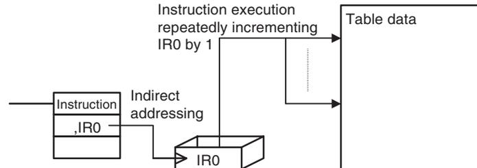
The Index operation uses the following procedure.
