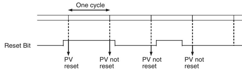
**Note** The comparison operation can be set to stop or continue when a high-speed counter is reset. This enables applications where the comparison operation can be restarted from a counter PV of 0 when the counter is reset.
