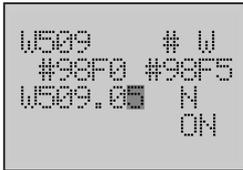
14. Use the **Up** button to change the bit address to **05**.
