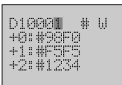
6. Use the **Forward** button to move the column cursor to the digit to be set. Use the **Up** button to change the leading word address to **10001**.
