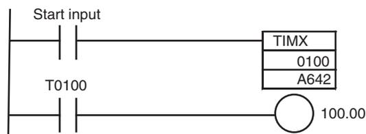
**Note** Set values from the analog adjuster may vary with changes in the ambient temperature and the power supply voltage. Do not use it for applications that require highly precise set values.
