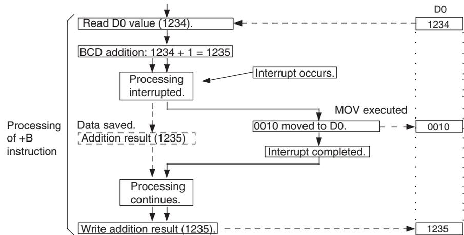
The interrupt occurs during processing of the +B instruction and the result is saved temporarily without being written to the destination word (D0).
