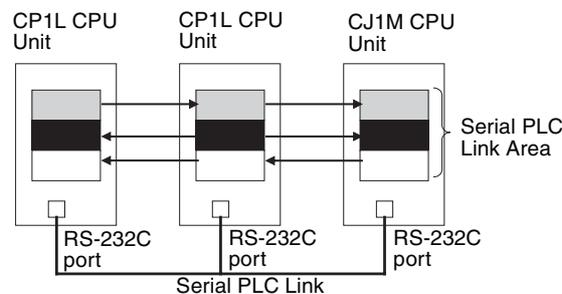
Addresses not used for Serial PLC Links can be used in programming, the same as the Work Area.
