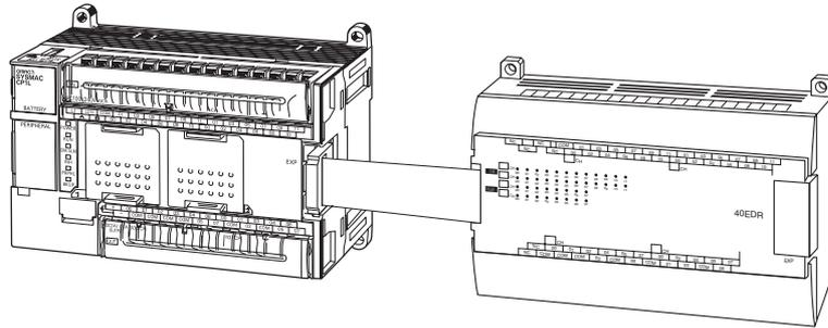
3. Replace the cover on the CPU Unit's or the Expansion I/O Unit's expansion connector.
