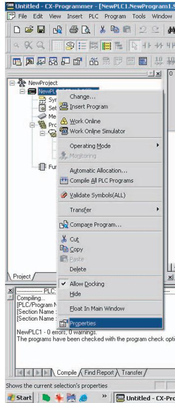
2. Select the **Execute Timer/Counter as Binary** Option in the PLC Properties Dialog Box. The timers and counters for all tasks will be executed in binary mode.
