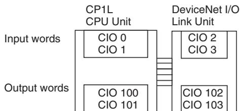
All of the words allocated to the DeviceNet I/O Link Unit are used to read and write data between the CPU Unit of the DeviceNet I/O Link Unit and the CPU Unit of the DeviceNet master, as shown in the following illustration.
