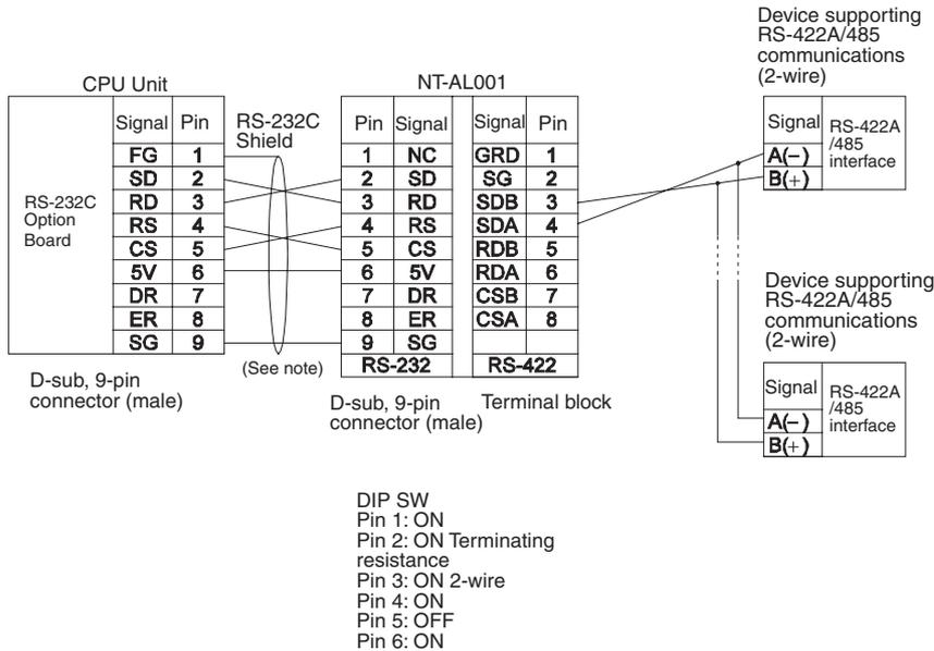
**Note** We recommend using the following NT-AL001 Link Adapter Connecting Cables to connect to NT-AL001 Link Adapters.
