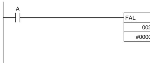
When execution condition A goes ON, an error with FAL number 002 is generated, A402.15 (FAL Error Flag) is turned ON, and A360.02 (FAL Number 002 Flag) is turned ON. Program execution continues.
