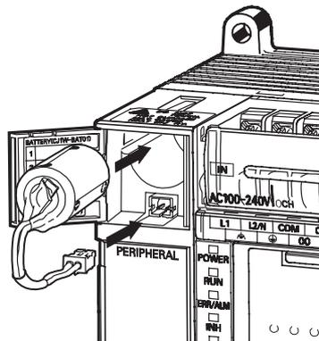
**⚠ WARNING** Never short-circuit the battery terminals; never charge the battery; never disassemble the battery; and never heat or incinerate the battery. Doing any of these may cause the battery to leak, burn, or rupturing resulting in injury, fire, and possible loss of life or property. Also, never use a battery that has been dropped on the floor or otherwise subject to shock. It may leak.
