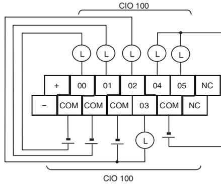
AC-power-supply models have a 24-VDC output terminals (+/-) on the lower terminal block. They can be used as a DC power supply for the input circuit.
