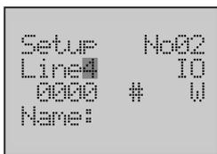
3. Enter the User Monitor Setup Screen 2, line 4. User settings backed up in EEPROM are replaced by default settings. Then reset the screen.
