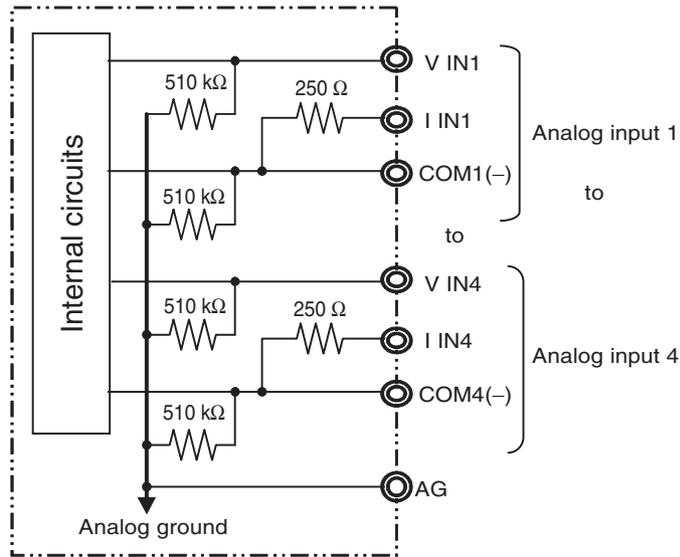
■ Wiring for Analog Inputs
