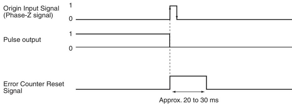
When the Origin Proximity Input Signal is received, the motor will begin decelerating from the origin search high speed to the origin search proximity speed. In this operating mode, the motor will stop at the Origin Input Signal after deceleration is completed.
