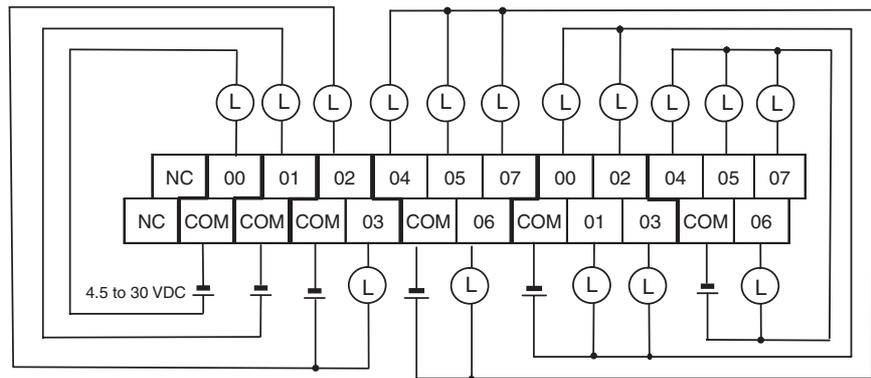
**CP1W-40EDT1/CPM1A-40EDT1 (Sourcing Transistor Outputs)**
