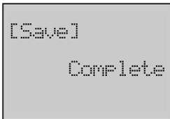
9. When the rate comes up to 100%, the saving is finished. Then it will display a complete screen.
