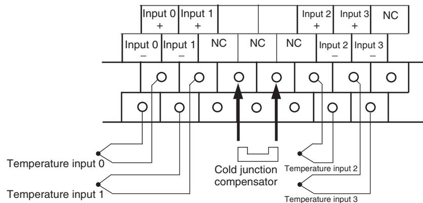
**Note** When using a Temperature Sensor Unit with a thermocouple input, observe the following precautions:
