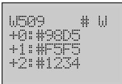
18. Press the **OK** button to save the setting. Press the **ESC** button to return to the previous screen. Then the data on W509 displayed in the Monitor Screen will be 98D5.
