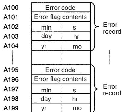
The following data would be generated in an error record if a memory error (error code 80F1) occurred on 1 April 1998 at 17:10:30 with the error located in the PLC Setup (04 hex).
