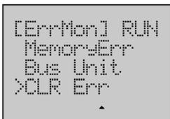
10. If the memory error itself has not been eliminated, when the Error Monitor Screen is updated, the error will be displayed again in the screen.
