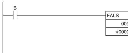
When execution condition B goes ON, an error with FALS number 003 is generated, and A401.06 (FALS Error Flag) is turned ON. Program execution is stopped.
