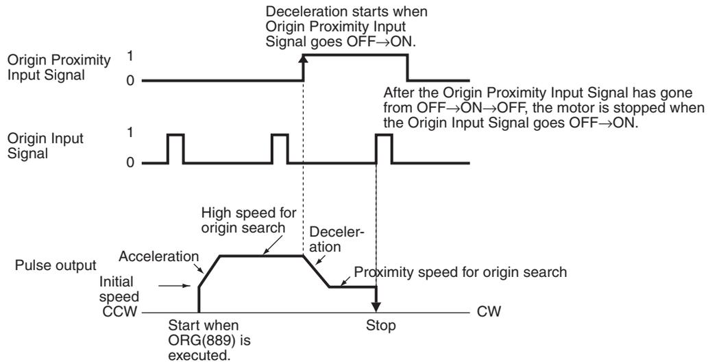
**Origin Detection Method 2: Origin Proximity Input Signal Reversal Not Used**
