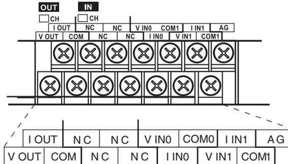
**Note** For current inputs, short V IN0 to I IN0 and V IN1 to I IN1.
