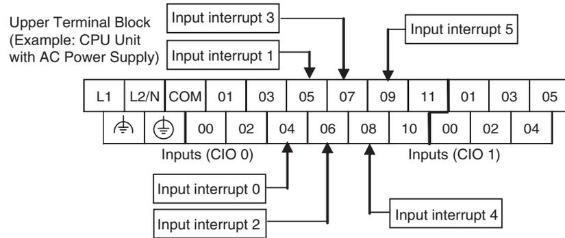
**Input Terminal Block of CPU Units with 40 I/O Points**
