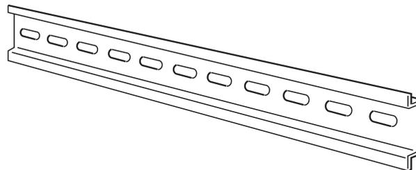
Secure the DIN Track to the control panel using M4 screws separated by 210 mm (6 holes). The tightening torque is 1.2 N-m.
