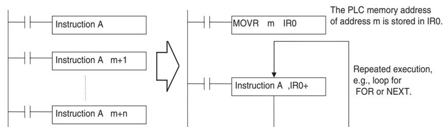
If, for example, instruction A above is a comparison instruction, table data could be read from start to the end of the table to compare all of the data with a specific value. In this way, blocks of user-defined processing can be freely created depending by applying Index Registers.
