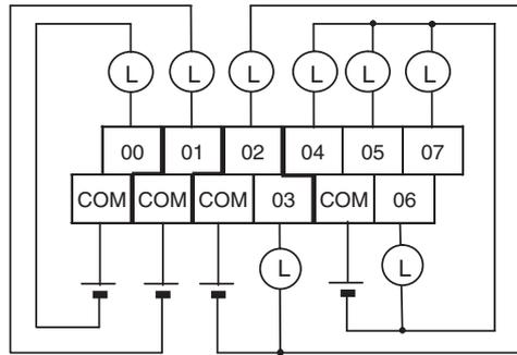
**16-point Output Units (CP1W/CPM1A-16E□□) (Terminal Block is not Removable)**
