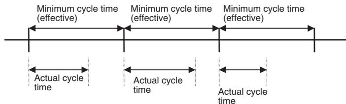
This setting is effective only when the actual cycle time is shorter than the minimum cycle time setting. If the actual cycle time is longer than the minimum cycle time setting, the actual cycle time will remain unchanged.
