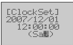
7. Use the **Forward** button to move the column cursor to the position of PLC week. Use the **Down** or **Up** button to select **Sat**.
