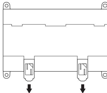
2. Lower the Units so that they catch on the top of the DIN Track, and then press them forward all the way to the DIN Track at the bottom.
