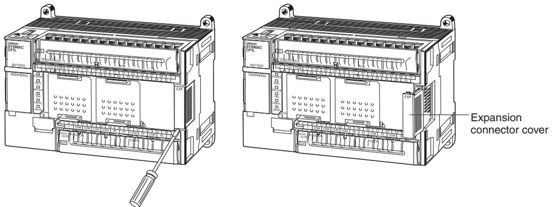
2. Insert the Expansion I/O Unit's connecting cable into the CPU Unit's or the Expansion I/O Unit's expansion connector.
