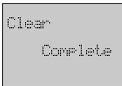
8. When the rate comes up to 0%, the clearing is finished. Then it will display a complete screen.
