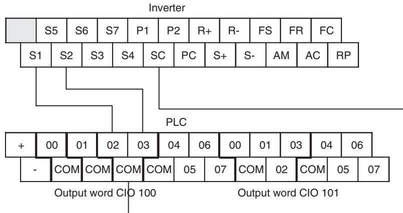
CP1W/CPM1A-DA041 (Current Output) Connections to Inverter
