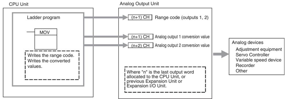
1. Connecting the Analog Output Unit
