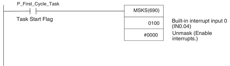
**Built-in Input 0 Interrupt Task (Interrupt Task 140)**
