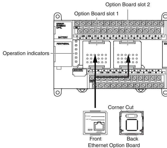
**Note** If two CP1W-CIF41 (unit version 1.0) Ethernet Option Boards are mounted on the CP1L/CP1H PLC, the CP1W-CIF41 mounted on Option Board slot1 (left side) will run in abnormal status and ERR indicator will be ON. If the ladder program operates the with CP1W-CIF41 fatal error, the PLC will generate the non-fatal error.
