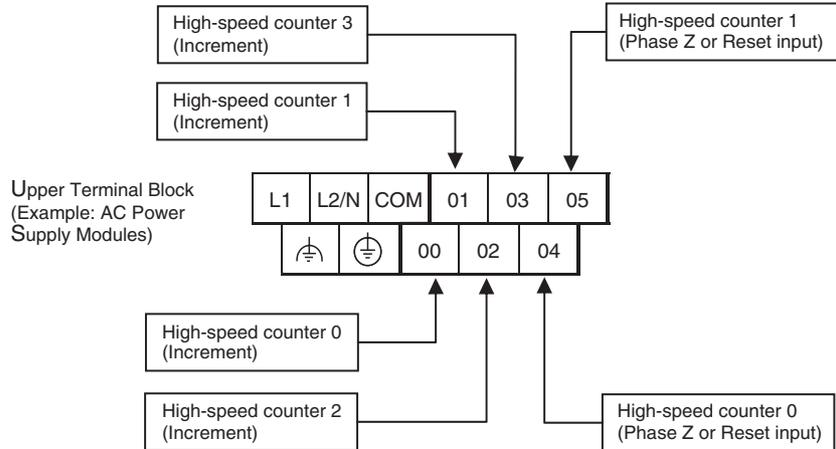
Input Terminal Arrangement for CPU Units with 14 I/O Points
