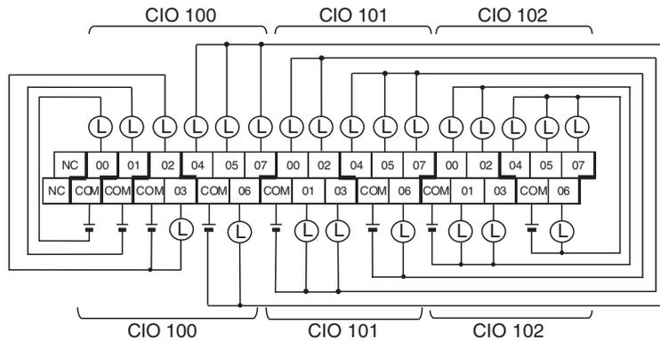
**3-5-2 I/O Wiring for CPU Units with 40 I/O Points**
