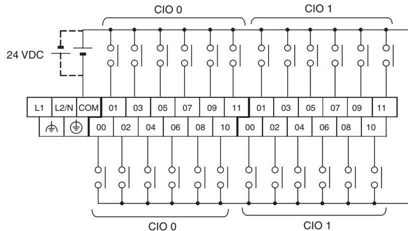
**Output Wiring (Lower Terminal Block, Removable)**
