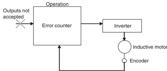
**Referencing the Automatically Calculated Inverter Frequency Command Value**
