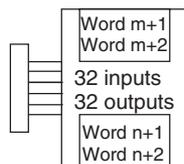
In the following example, a CompoBus/S I/O Link Unit is connected as the first Unit after the CP1L CPU Unit.
