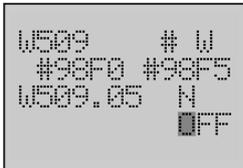
17. Press the **Down** or **Up** button to select the bit state **OFF**.
