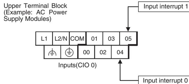
**Input Terminal Block of CPU Units with 14 I/O Points**
