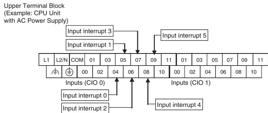
**Input Terminal Block of CPU Units with 60 I/O Points**
