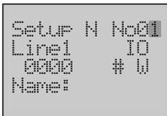
4. Press the **OK** button to enter the User Monitor Setup Screen.
