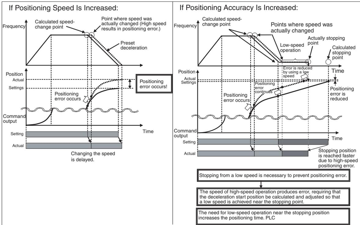
**Inverter Positioning with the CP1L**
