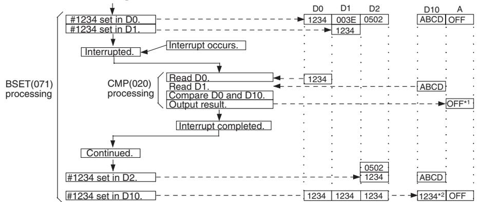
Since the interrupt occurs during BSET(071) processing and before #1234 is set in D10, the content of D0 and D10 do not match when the comparison is made in the interrupt task (\*1) and output A remains OFF.
