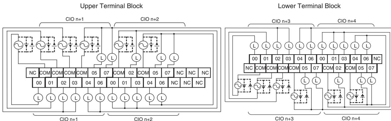
**Output Wiring CP1W-32ET (Sinking Transistor Outputs)**
