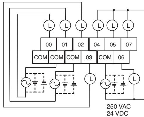
**CP1W-20EDT/CPM1A-20EDT (Sinking Transistor Outputs)**
