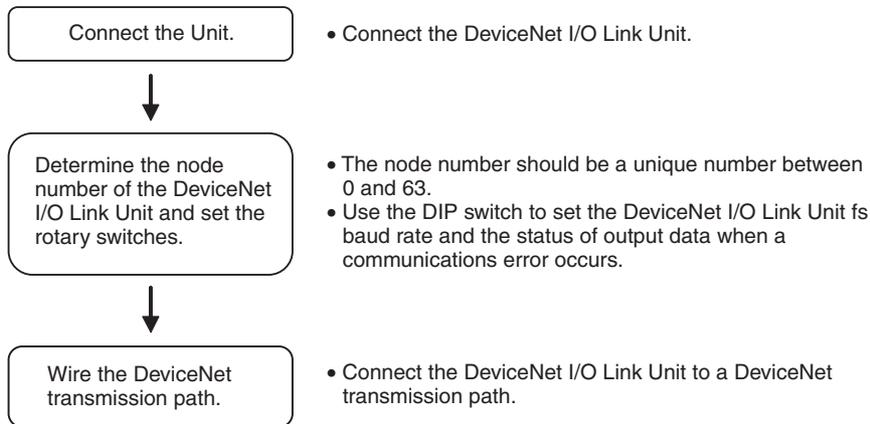
**Connecting the DeviceNet I/O Link Unit**
