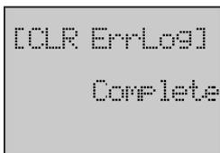
10. Press the **OK** button to clear the error history. When the clearing is finished, it will display a complete screen.
