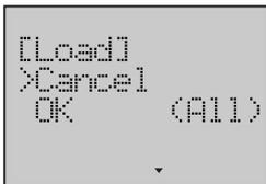
4. Press the **OK** button to enter the Load Operation Screen. Select the operation mode in the following table.
