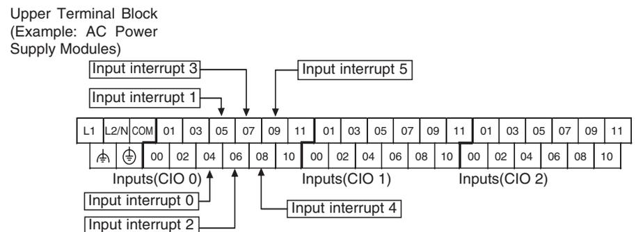
**Setting the Input Functions in the PLC Setup**
