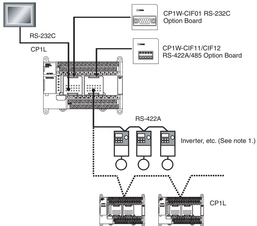
**Note** (1) The Modbus-RTU easy master (available for all models) makes it easy to control Modbus Slaves (such as Inverters) with serial communications. After the Modbus Slave address, function, and data have been preset in
