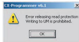
3. If an incorrect password is input five times consecutively, read protection will not be released even if the correct password is input on the sixth attempt and displaying and editing the entire user program or the specified tasks will be disabled for two hours.
