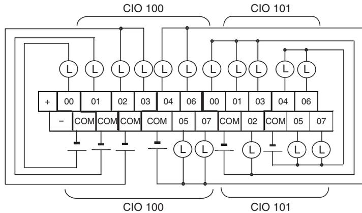
AC-power-supply models have a 24-VDC output terminals (+/-) on the lower terminal block. They can be used as a DC power supply for the input circuit.
