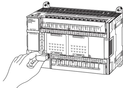
2. Holding the Memory Cassette with the side with the nameplate facing upwards, insert the Memory Cassette all the way into the slot.
