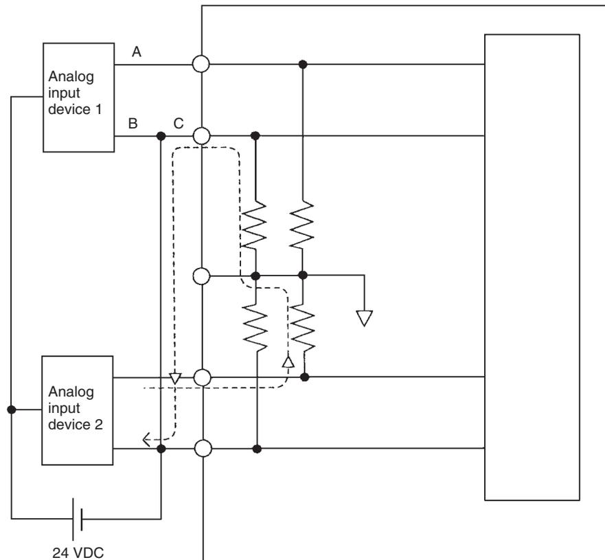
Example: If analog input device 2 is outputting 5 V and the same power supply is being used for both devices as shown above, approximately 1/3, or 1.6 V, will be applied to the input for input device 1.
