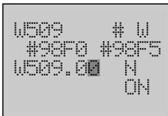
8. Press the **Forward** button to move the column cursor to the digit to be set. Use the **Down** or **Up** button to change the data to **12345678**.
