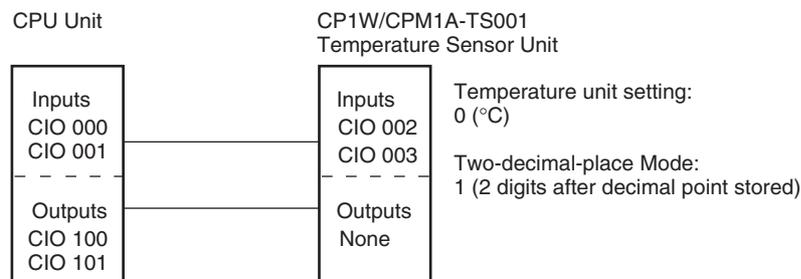
In this example, 100 times the temperature data for temperature input 0 is stored in binary form in D100 to D102.
