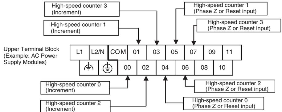
Input Terminal Arrangement for CPU Units with 30 I/O Points
