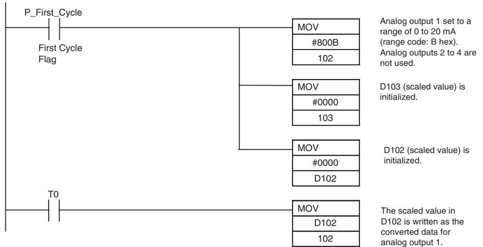
Refer to the first line in the programming example in *Referencing the Automatically Calculated Inverter Frequency Command Value* on page 334 for a timer for the time required for the Analog Output Unit's data to be valid (analog conversion trigger: T0).
