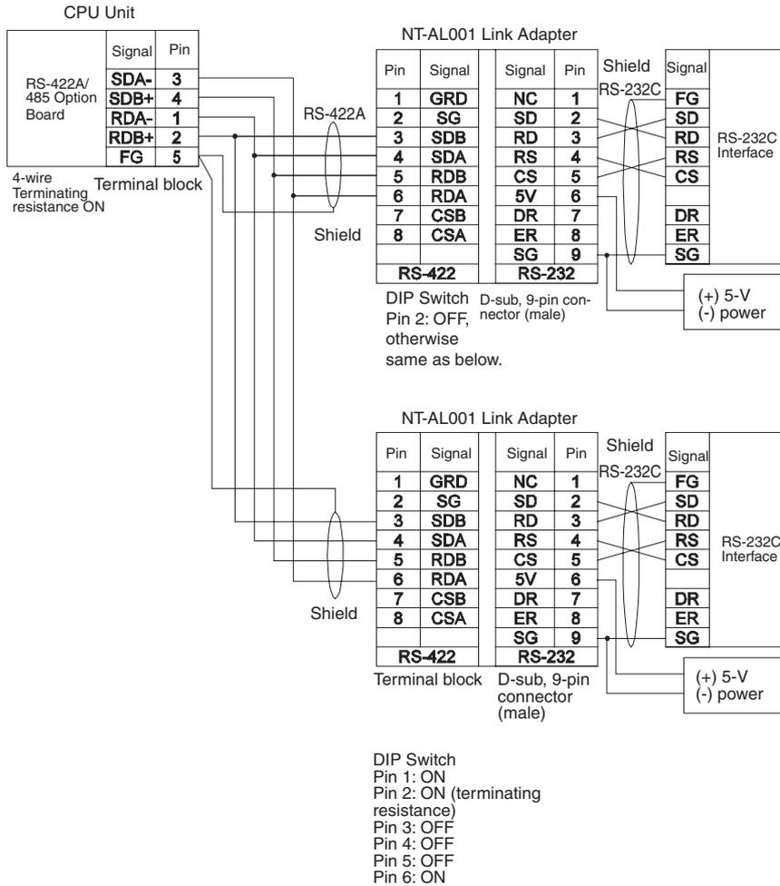
**1:N NT Link Connections with Programmable Terminals**
