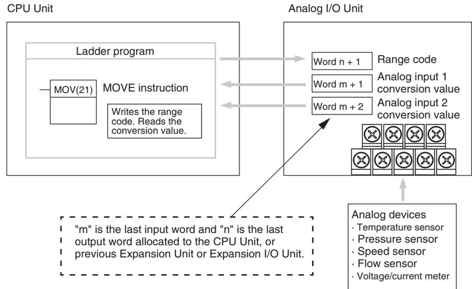
"m" is the last input word and "n" is the last output word allocated to the CPU Unit, or previous Expansion Unit or Expansion I/O Unit.
