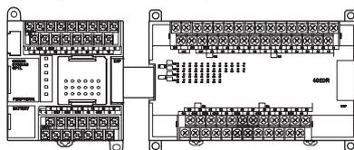
One CP-series Expansion I/O Unit or Expansion Unit can be added.
