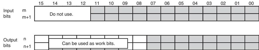
Two input words (24 bits) and two output words (16 bits) are allocated to a 40-point Expansion I/O Unit. Input bits 12 to 15 cannot be used as work bits. Output bits 08 to 15, however, can be used as work bits.
