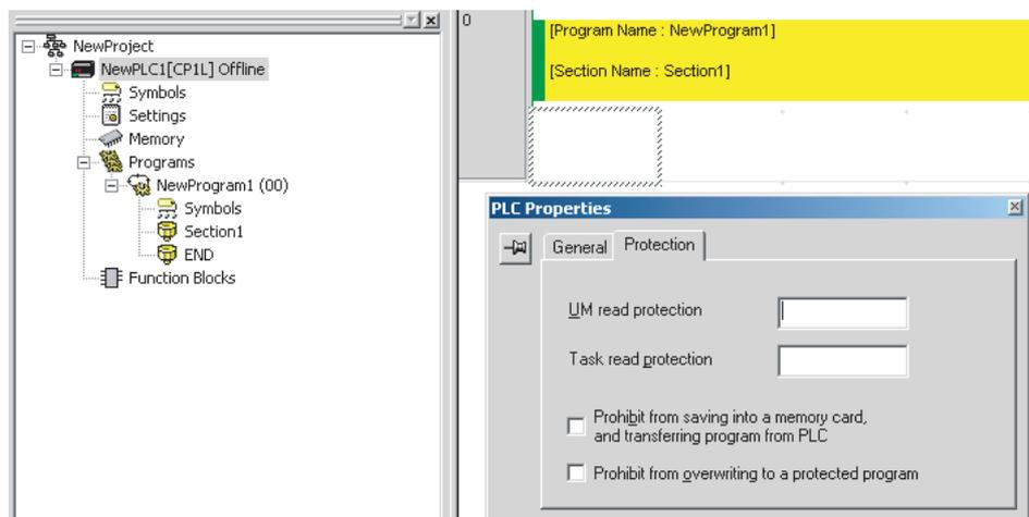
3. Connect online and select **PLC - Transfer - To PLC** to transfer the program. The tasks registered in step 2 will be password-protected.
