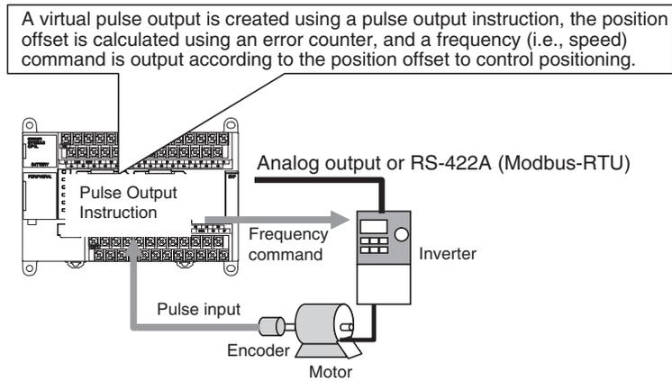
**Note** If high-precision positioning is required, we recommend using an inverter with vector control.
