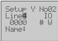
6. Use the **Forward** button to move the column cursor to the Line No. position.
