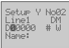
11. Use the **Forward** button to move the column cursor to the memory address position.
