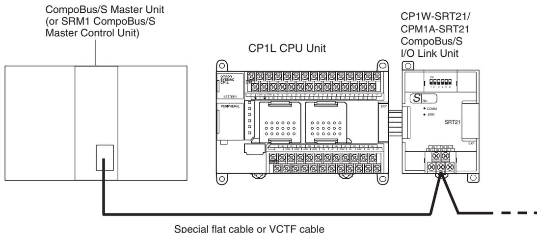
From the standpoint of the CP1L CPU Unit, the 8 input bits and 8 output bits allocated to the CompoBus/S I/O Link Unit are identical to input and output bits allocated to Expansion I/O Units even though the CompoBus/S I/O Link Unit does not control actual inputs and outputs. The input and output bits allocated to the CompoBus/S I/O Link Unit are one side of an I/O link between the slave CPU Unit and the CPU Unit to which the Master Unit is connected.
