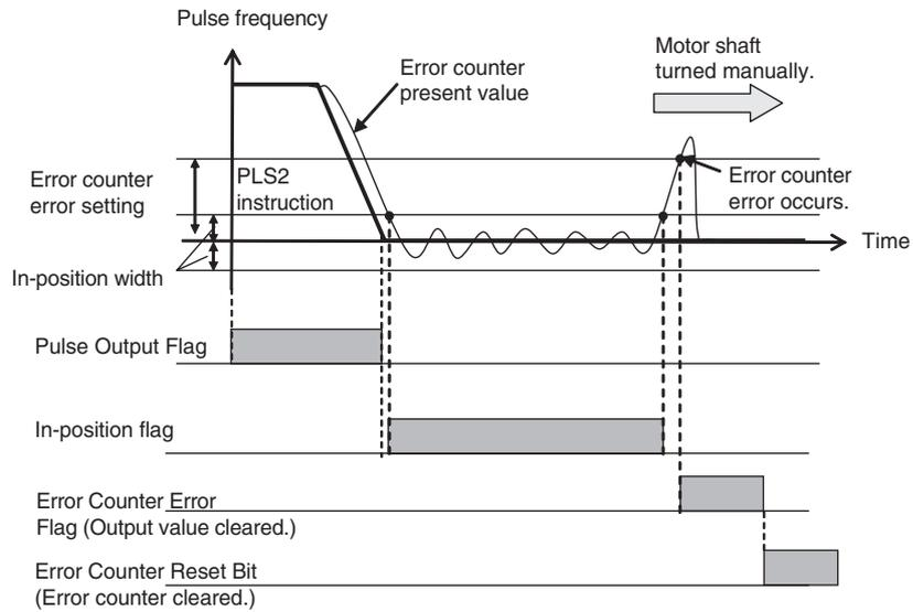
**Low-speed Operation Using Minimum Output Setting**
