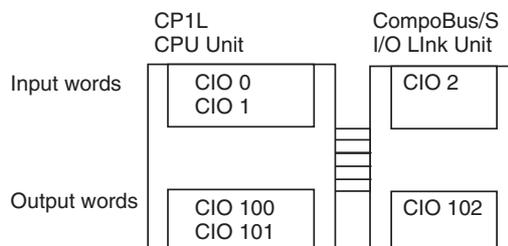
The input word (m+1) contains the 8 bits of data from the Master Unit and two CompoBus/S communications flags.
