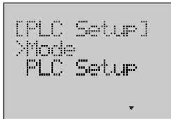
3. Press the **OK** button to enter the PLC Setup menu.
