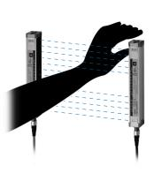
For presence inspection with a horizontal installation, types with minimum detectable object sizes of 40 mm (optical axis pitch: 30 mm) and 70 mm (optical axis pitch: 60 mm) can also be manufactured. (Please contact your OMRON Representative.)
