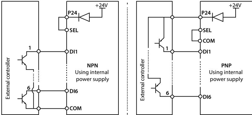
Figure 4-8 Connection when using internal 24V power supply
