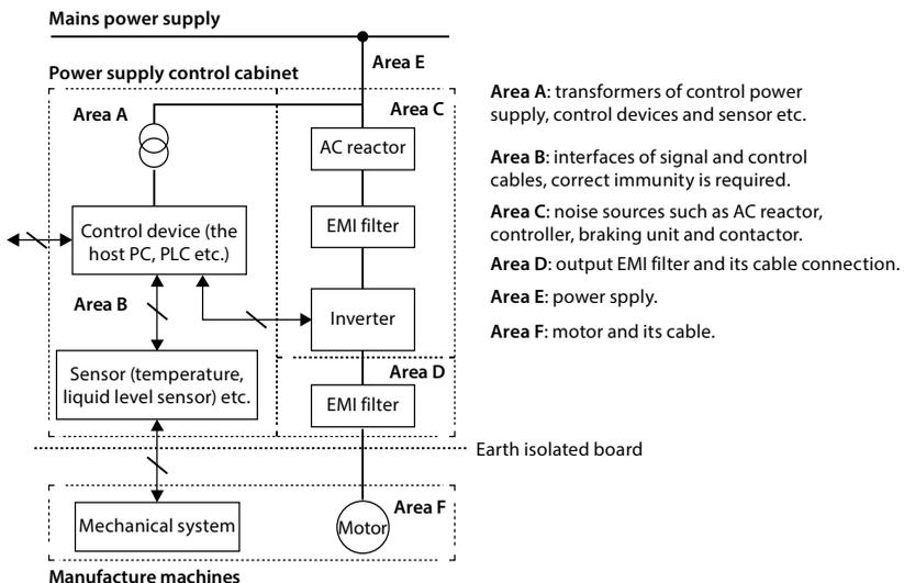
Figure 4-15 System wiring
