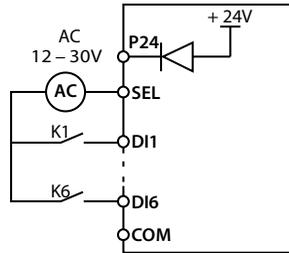
Figure 4-9 Connection when AC signal inputs (7.5 - 75kW)
