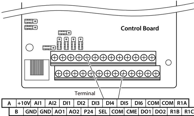
Figure 4-1 Control board terminal (7.5 - 75kW)
