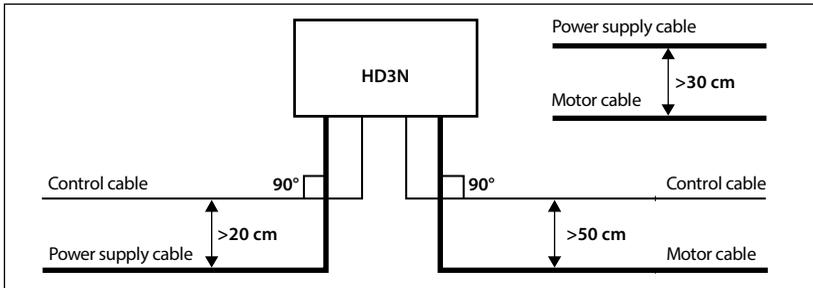
Figure 4-16 System wiring
