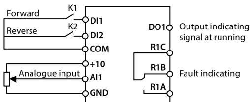
2. Power on, and set function code according to connection.
