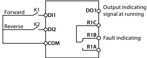
2. Power on HD3N. Set function codes according to connection.
