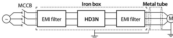
Figure 4-20 Reducing RF interference
