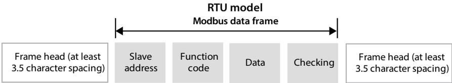
MODBUS adopts “Big Endian” encoding mode, higher byte prior to lower byte at sending.
