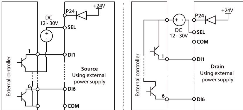
Figure 4-7 Source / Drain connection when using external power
