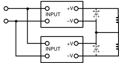
When connecting the power supplies in series with an operation amplifier, connect diodes to the output terminals (as shown by the dotted lines in the figure). Contact your OMRON representative for details on connecting diodes.
