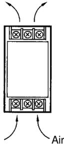
When mounting two or more power supplies side-by-side, allow at least 10 mm spacing between them, as shown in the following diagram.
