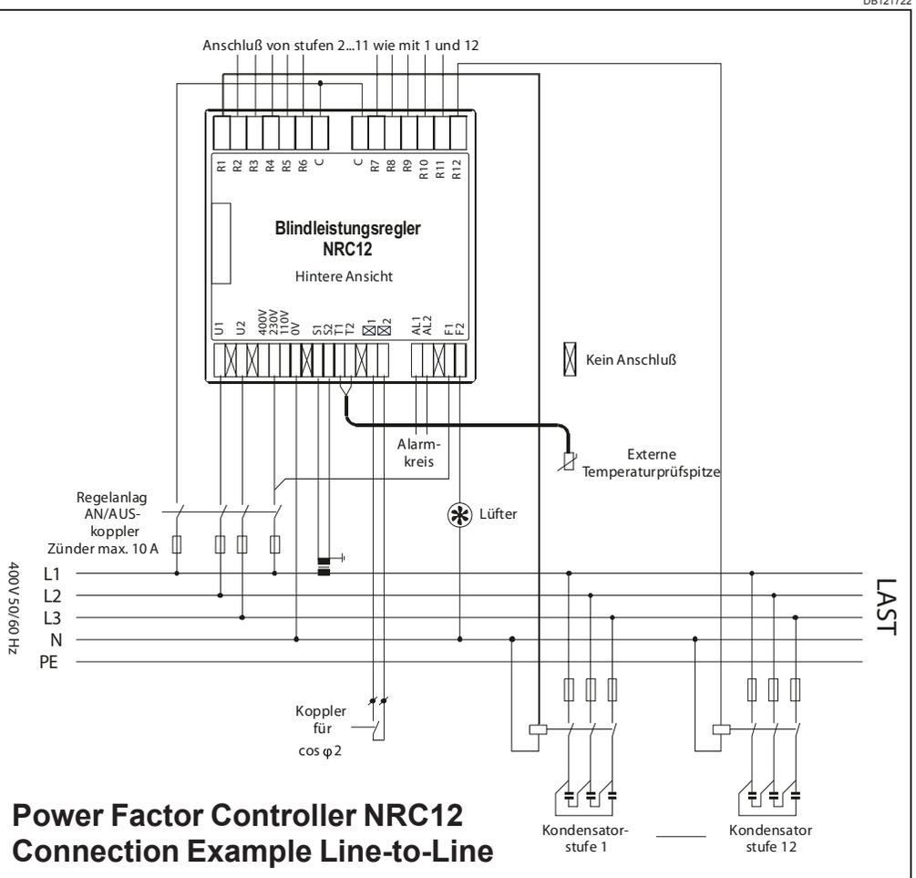
Figure 1-1: Controller connection example Line-to-Line (LL)
