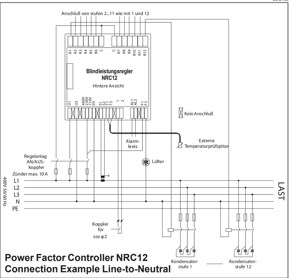
Figure 1-2: Controller connection example Line-to-Neutral (LN)
