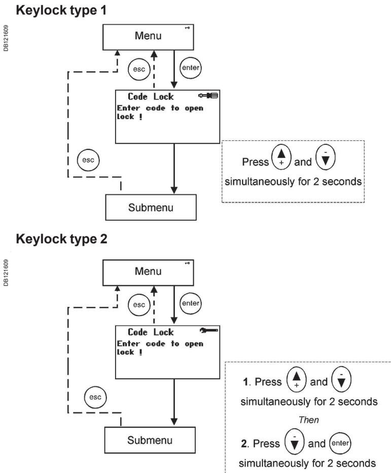
Figure 4: Entering a submenu with a keylock.
