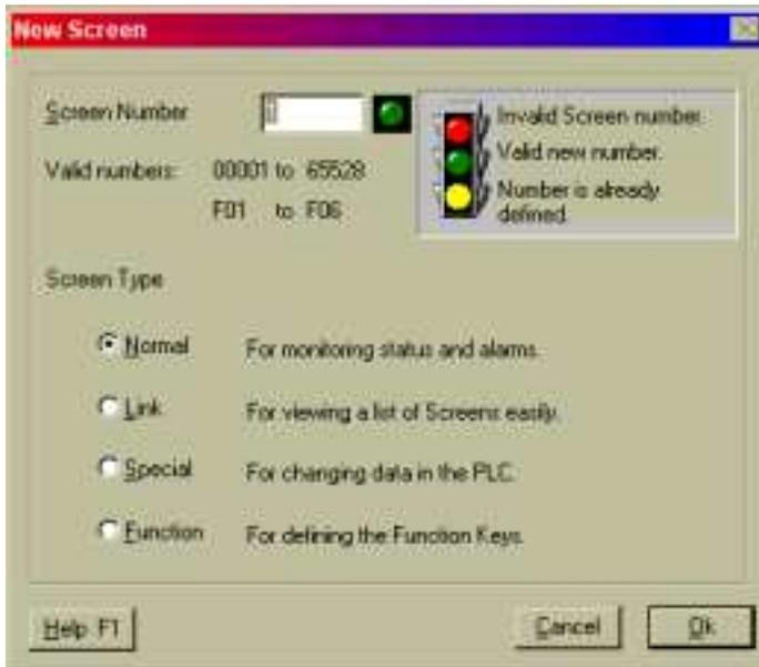
3. Four different types of screens can be selected from the New Screen dialog: Normal, Link, Special, and Function. The following sections will discuss each type of screen. Choose a screen type, enter a screen number, and select OK to launch the Editing Screen dialog.
