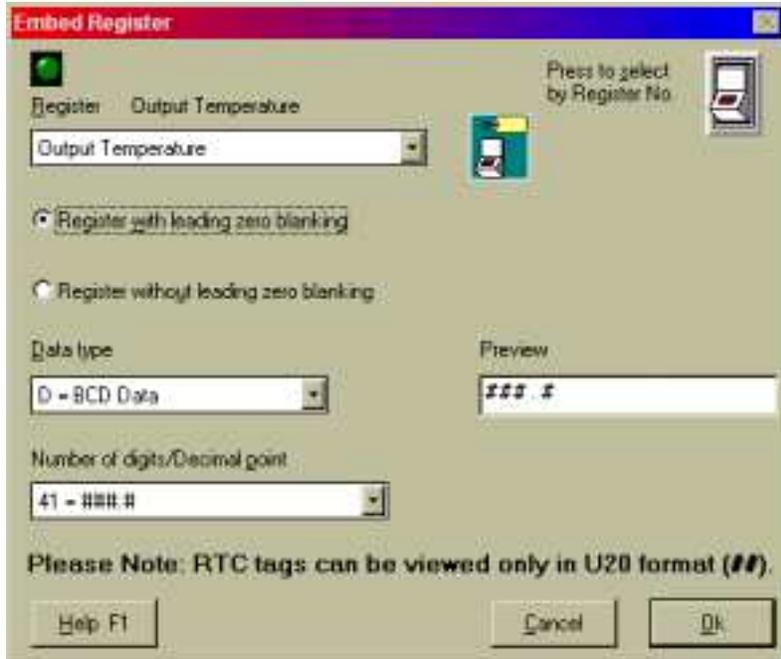
Once the register is assigned and formatted, select OK. Text placeholders will appear in the display window at the cursor location. These placeholders can be positioned by adding characters before the placeholders.
