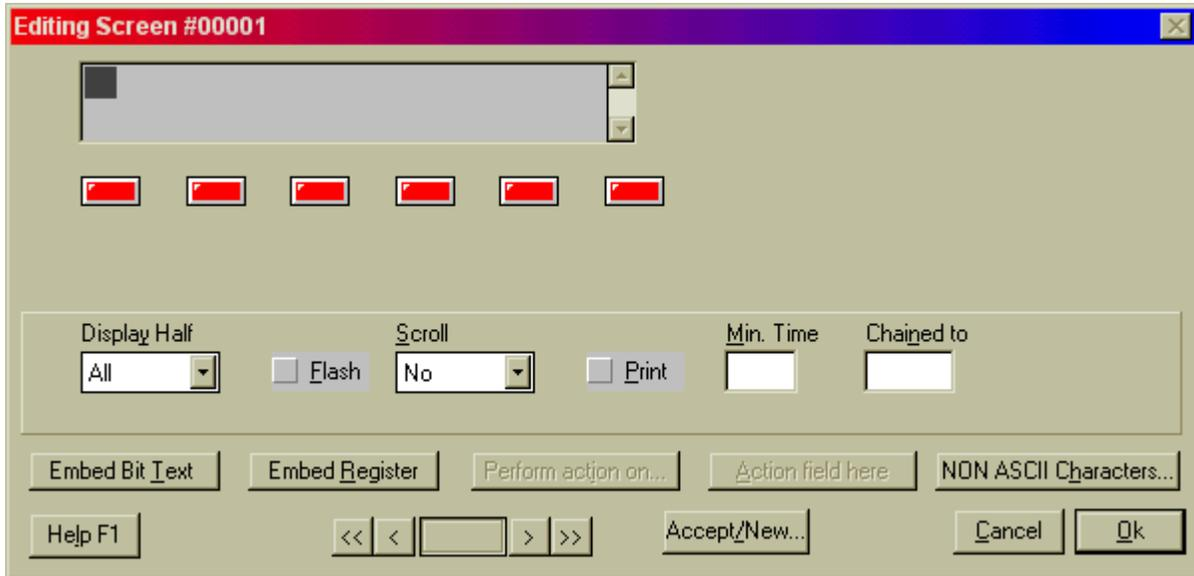
The text window in the upper left corner represents the NT2S display window. Some Normal screen settings include:
