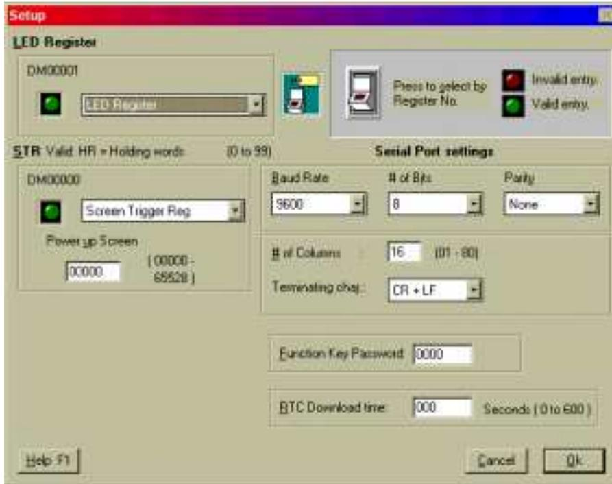
**LED Register** – This setting tells the NT2S which TAG to reference for the LED Register. Any TAG of the proper type can be referenced for this setting. The default TAG is labeled “LED Register”.
