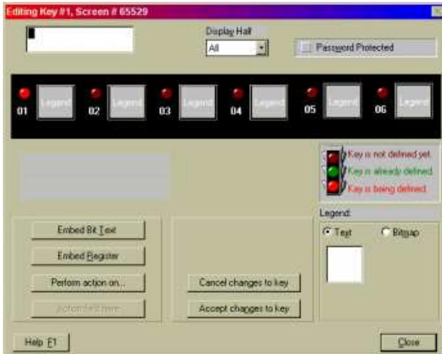
Programming begins by clicking on the function key that requires programming. Configure the action of the function key by clicking on PERFORM ACTION ON button.
