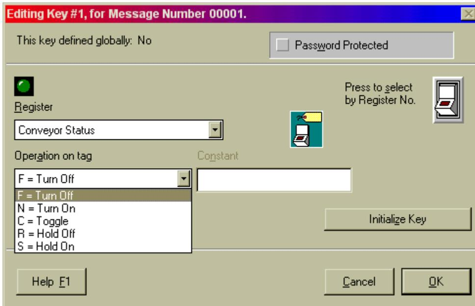
Bits can be controlled in several ways. *Turn Off* and *Turn On* functions force set the bit to the 0 or 1 position. *Toggle* alternates the bit between 1 and 0 as the function key is pressed. *Hold Off* and *Hold On* set the bit to a 0 or a 1 as long as the function key is held (momentary switch).
