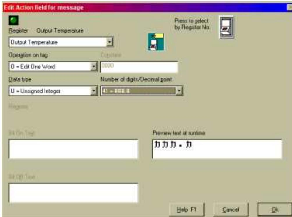
Operations can be performed on register or coil tags. (Recommend using Special screens only for changing registers, not coils. Use the function keys of a normal screen for changing coils.)
