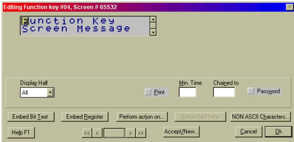
Click on the PERFORM ACTION ON button to change global function key program. Enter MIN TIME to control the time of display of function key message.
