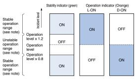
Note: If the operation level is set to the stable operation range, the E3G will operate with the highest reliability and without being influenced by temperature change, voltage fluctuation, dust, or setting change.
