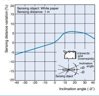
Sensing Object Angle (Left and Right)
