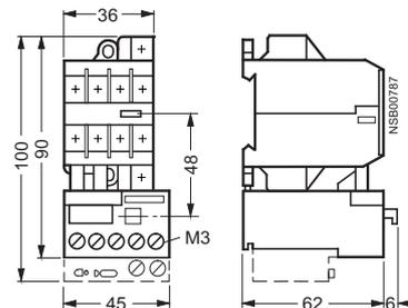
**3RT19 16-4BB41** links for paralleling, 4-pole, with terminal
