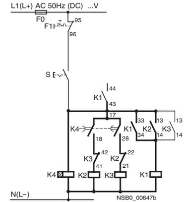
The contact element 17/18 is only closed in the wye stage; the contact element is open in the delta stage as well as in the de-energized state. S1 (S) is connected to clamping point K1/33.
