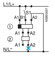
A2 must only be connected to N(L-) from the timing relay.
