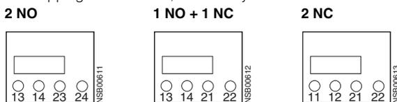
3RH19 21-.FE22 solid-state compatible auxiliary switch block, 4-pole,
