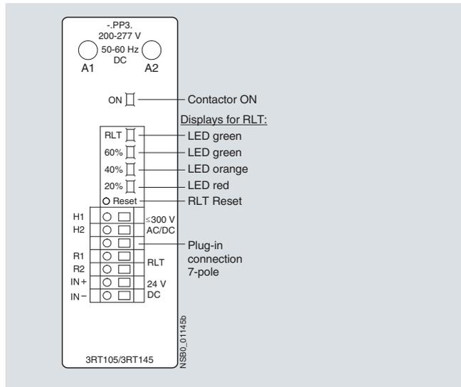
To supply the solenoid and the remaining lifetime indicator with power, the control supply voltage  $U_s$  must be connected to terminals A1/A2 of the laterally mounted solid-state module. The control inputs of the contactor are connected to a 7-pole plug-in connection; the screwless spring-type connection is part of the scope of supply.
