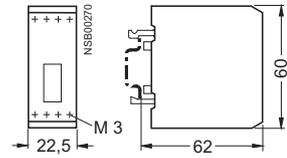
**3TX7 004, 3TX7 005 coupling links in double-decker design**
