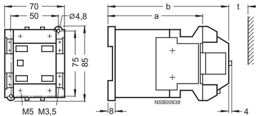
t = minimum clearance from insulated components: 15 mm (600 V and 750 V)
