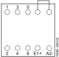
Series resistor  $R_V$  plugged on, NC contact prewired.
