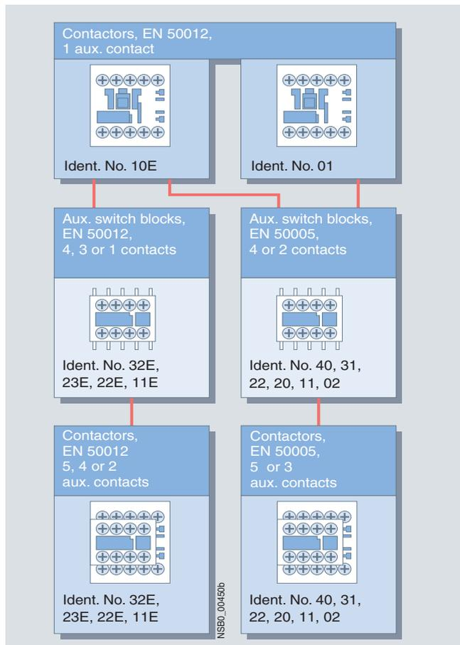
Size S00 contactors have an auxiliary contact integrated in the basic unit.
