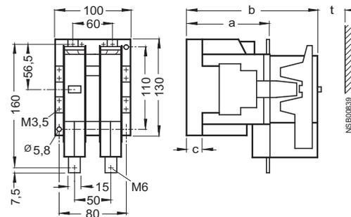
t = minimum clearance from insulated components: 15 mm (600 V),
