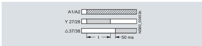
The contactor on which the solid-state, time-delay auxiliary switch block is mounted operates without a delay.
