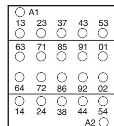
*Position of the terminals for 3RH1 contactor relays, size S00*
