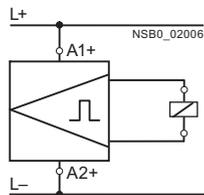
Circuit diagram for railway-type contactors with solid-state coil excitation
