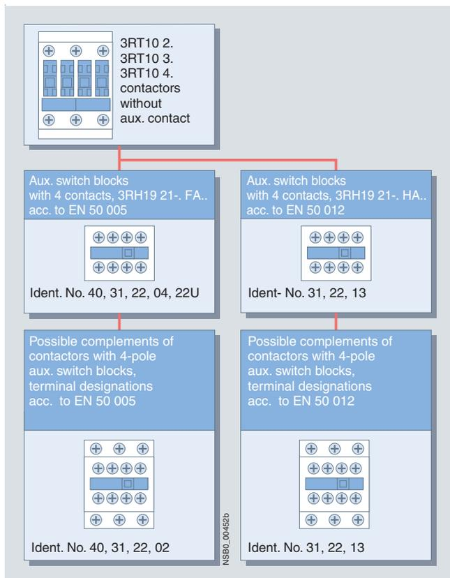
A diverse range of auxiliary switch blocks is available for various applications. The contactors themselves have no integrated conducting path.
