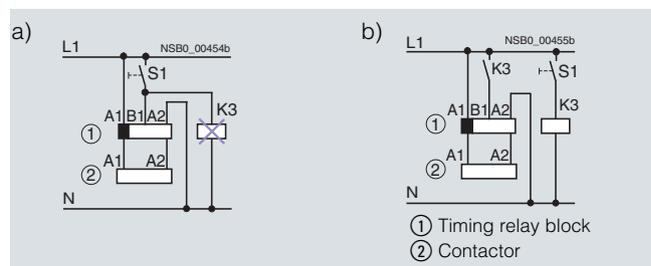
The activation of loads parallel to the start input is not permissible when using AC control voltage (see (a) in the circuit diagram).
