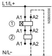
A2 can be connected to N(L-) using either the contactor or the timing relay. --- optionally connect
