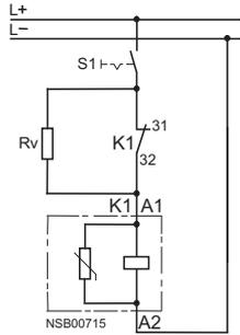
Circuit with series resistor R<sub>v</sub> and reversing contactor K2 (for K1 contactors size 8 or larger)
