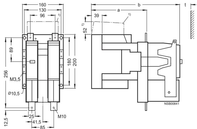
t = minimum clearance from insulated components: 25 mm (600 V and 750 V)
