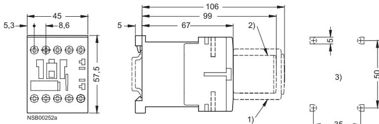
Lateral distance to grounded components = 6 mm
