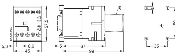
Deviating dimensions for coupling relays with Cage Clamp terminals:
