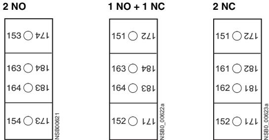
Second laterally mountable 3RH19 21-.KA.. auxiliary switch blocks (right)
