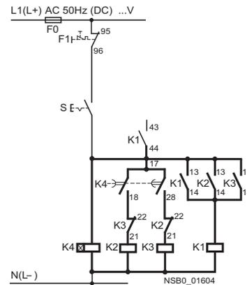
The contact element 17/18 is only closed in the wye stage; the contact element is open in the delta stage as well as in the de-energized state.
