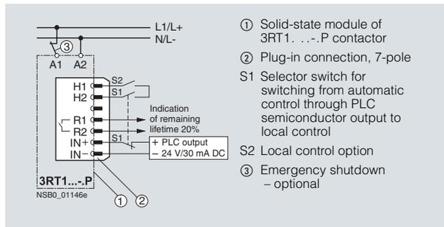
Possibility of switching from automatic control to local control by way of terminals H1/H2, i. e. automatic control through PLC or SIMOCODE/PROFIBUS DP can be deactivated e. g. at start-up or in the event of a fault and the contactor can be controlled manually.
