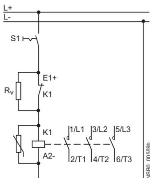
Series resistor  $R_v$  plugged on, NC contact prewired.
