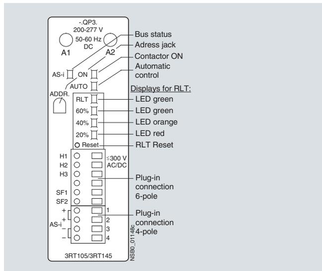
To supply the solenoid and the remaining lifetime indicator with power, the control supply voltage  $U_s$  must be connected to terminals A1/A2 of the laterally mounted solid-state module. The contactor itself is controlled by way of the integrated AS-Interface interface. The inputs and outputs are connected to a 10-pole plug-in connection; the screwless spring-type connections (6-pole for external connection and 4-pole for AS-Interface connection) are part of the scope of supply.
