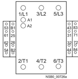
3TY7 561-1 . solid-state compatible auxiliary switch blocks for lateral mounting
