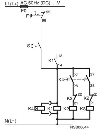
The contact element 27/28 for the solid-state time-delay auxiliary switch block with wye-delta function is only closed on the wye stage; the contact element is open in the delta stage as well as in the de-energized state.
