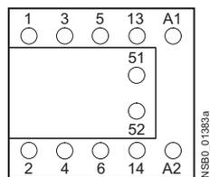
The auxiliary switch block contains 3 leading contacts (not shown), and one unassigned NO contact and one unassigned NC contact.
