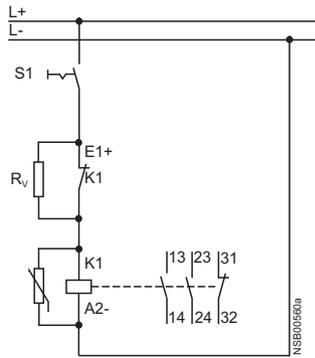
2 NO + 1 NC unassigned Series resistor  $R_v$  plugged on, NC contact prewired.
