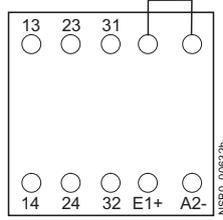
Series resistor  $R_V$  plugged on, NC contact prewired.
