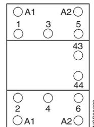
The auxiliary switch block contains 3 leading contacts (not shown) and one unassigned NO contact.
