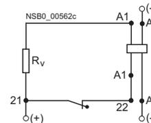
The series resistor is supplied separately packed. The 21/22 NC contact is necessary to wire the series resistor.
