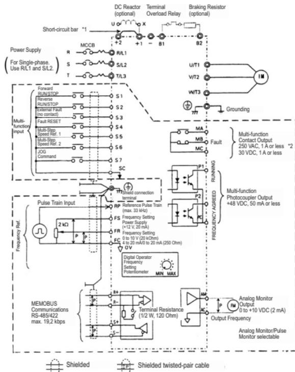
Only basic insulation (protective class 1, overvoltage category II) is provided for the control circuit terminals. Additional insulation may be necessary in the end product to conform to CE requirements.
