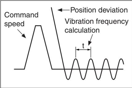
Measure the distance between the residual peaks (t), and calculate the vibration frequency (Hz) using the following formula.
