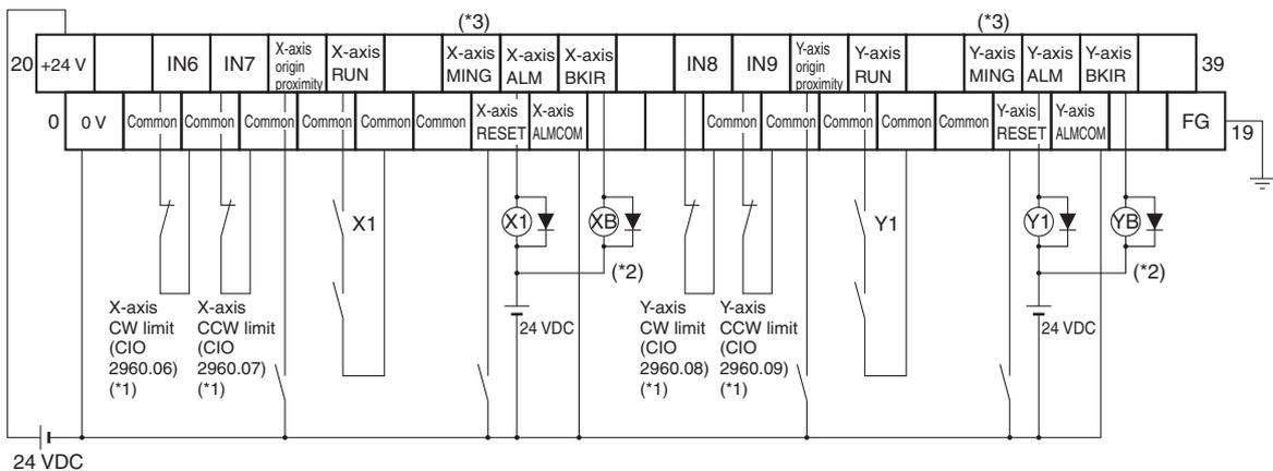
\*1. CW and CCW limit input signals can also be input through Input Units.
