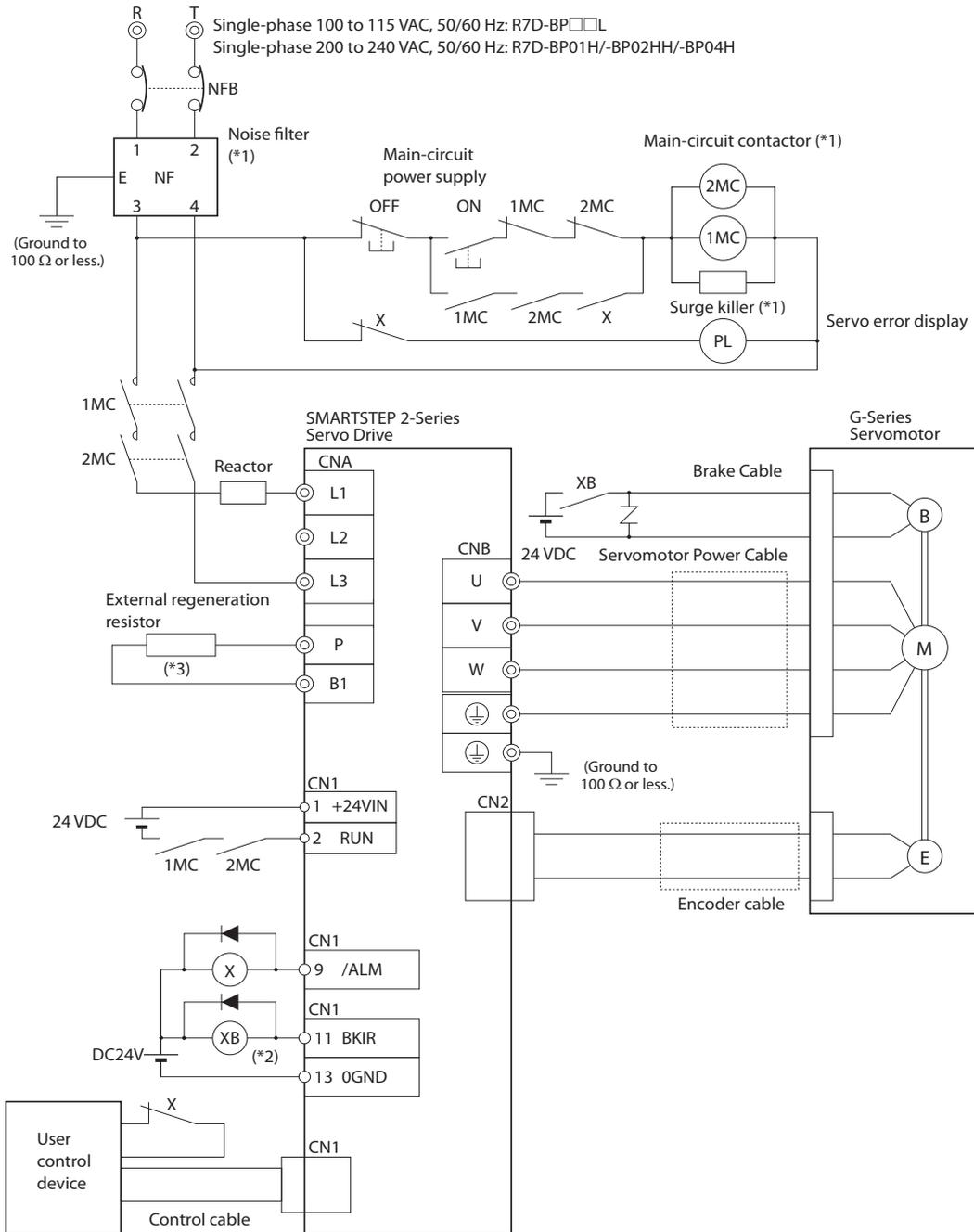
\*1. Recommended products are listed in 4-3 *Wiring Conforming to EMC Directives*.
