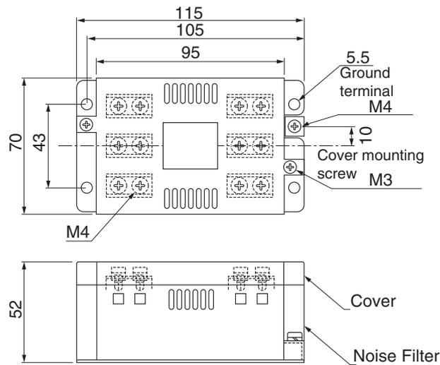
■ Noise Filter for the Brake Power Supply
