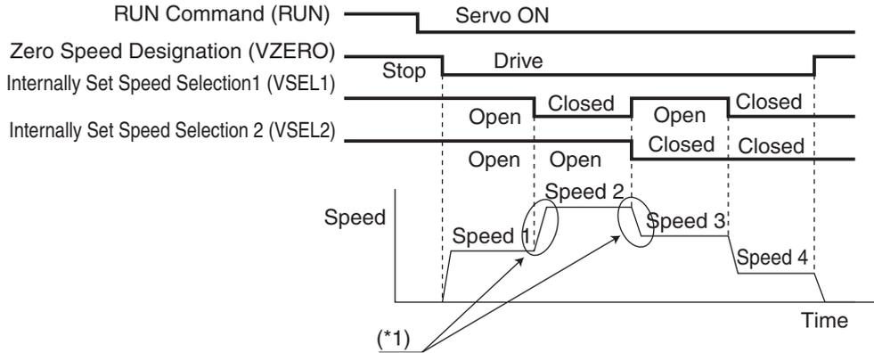
\*1. The acceleration time, deceleration time, and S-curve acceleration/deceleration time can be set using parameters (Pn58, Pn59, and Pn5A).
