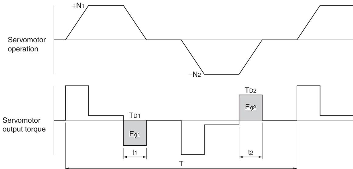
**Note** In the output torque graph, acceleration in the positive direction is shown as positive, and acceleration in the negative direction is shown as negative.
