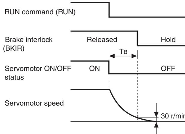
♦ “TB” in the above figure is the brake timing during operation (setting × 2 ms) or the time required until the Servomotor rotation speed falls to 30 r/min or lower, whichever is shorter.
