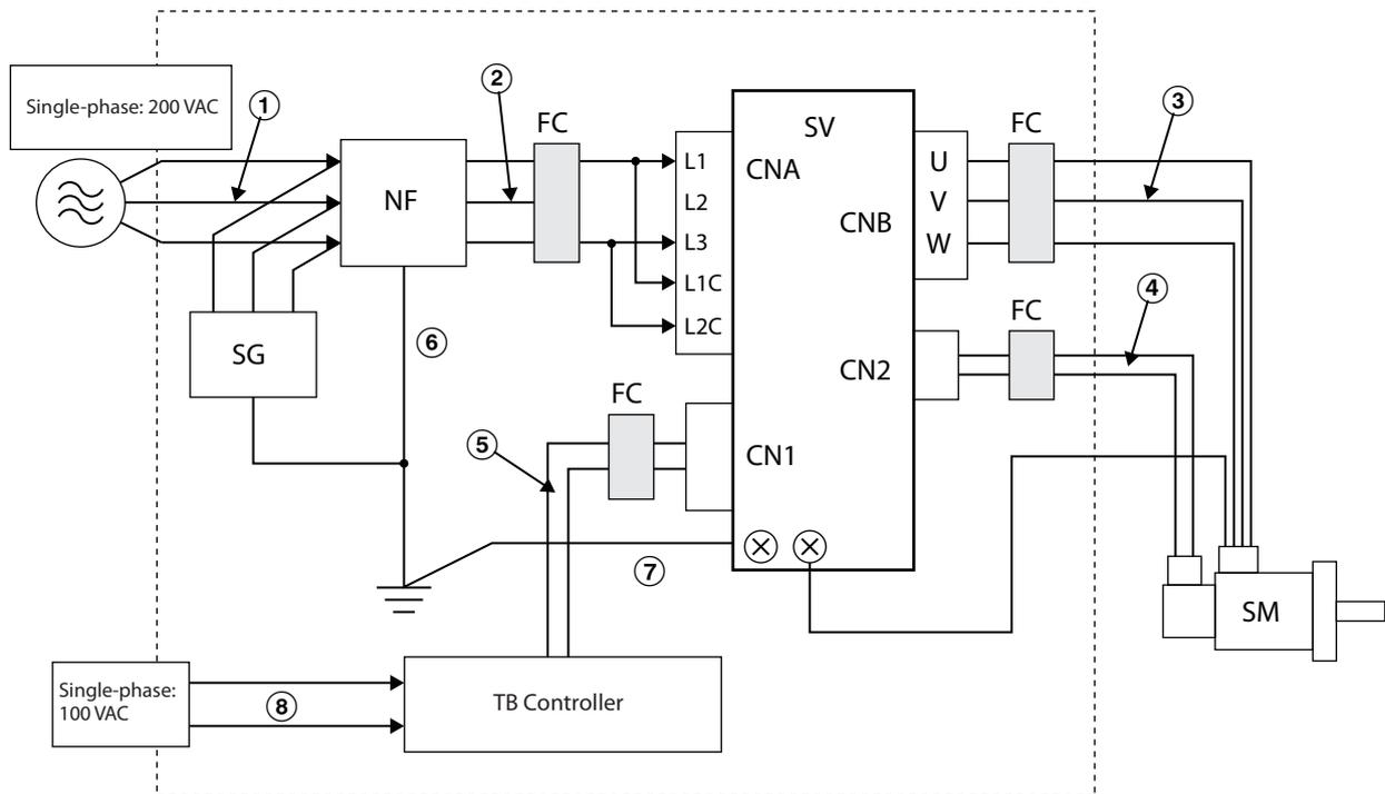
\*1. The main circuit power supply input terminals are L1 and L3.
