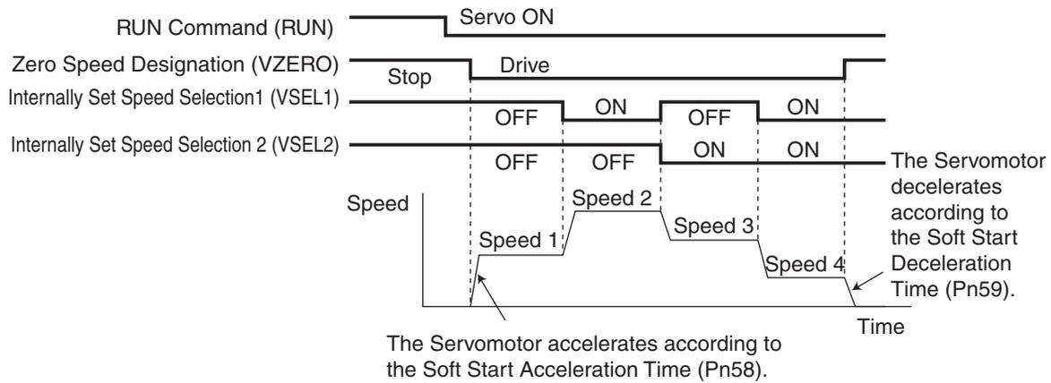
Parameter Block Diagram for Internally Set Speed Control Mode
