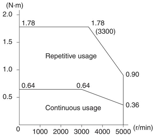
The following graphs show the characteristics with a 3-m standard cable and a 200-VAC input.
