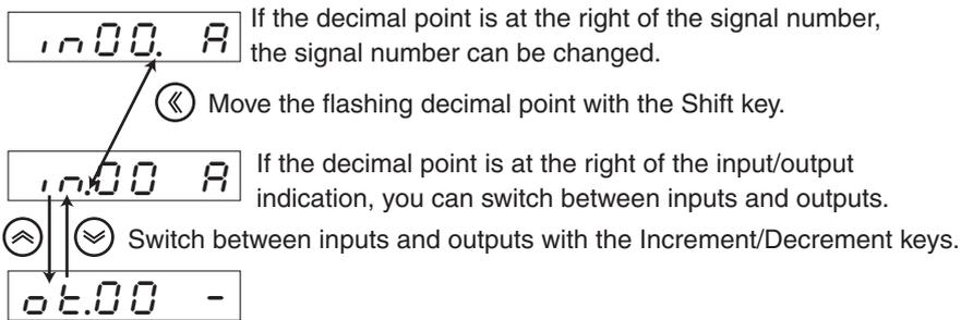
The following procedure can also be used to switch between input and output.
