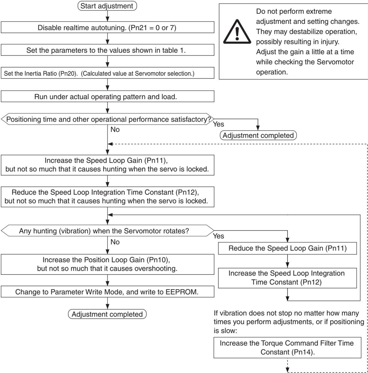
■ Adjustment in Internally Set Speed Control Mode
