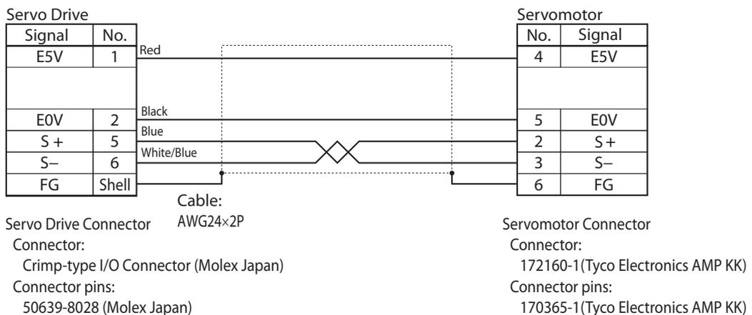
■ European Power Cable for Servomotors without Brakes (Flexible and Shielded Cables)
