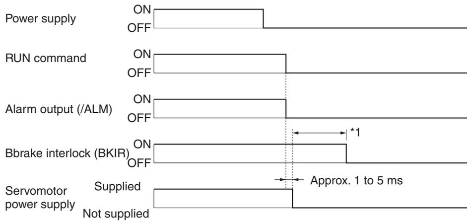
\*1. This time is the shorter value of either the setting for the Brake Timing during Operation (Pn6B) or the time it takes until the Servomotor rotation speed drops to 30 r/min or lower. Depending on the holding time of the power supply, this time may be shorter than the value set in Pn6B.
