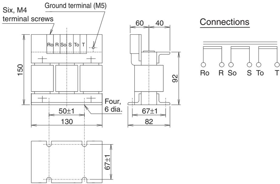
DIN Rail Mounting Unit Dimensions
