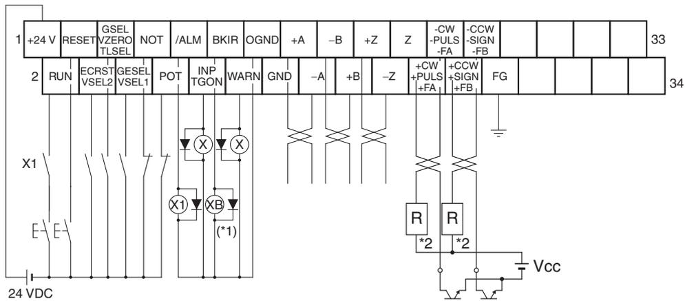
\*1. The XB contacts are used to turn the electromagnetic brake ON and OFF.
