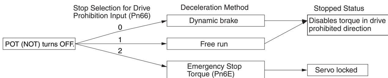
While the Forward Drive Prohibit Input (POT) is OFF, the Servomotor cannot be driven in the forward direction, but it can be driven in the reverse direction. Conversely, while the Reverse Drive Prohibit Input (NOT) is OFF, the Servomotor cannot be driven in the reverse direction, but it can be driven in the forward direction.
