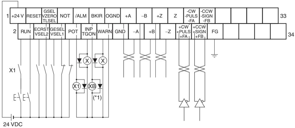
\*1. The XB contacts are used to turn the electromagnetic brake ON and OFF.
