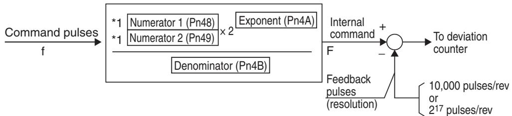
\*1. Numerator 1 or Numerator 2 is selected using the Electronic Gear Switch Input (GESEL: CN1 pin 28).
