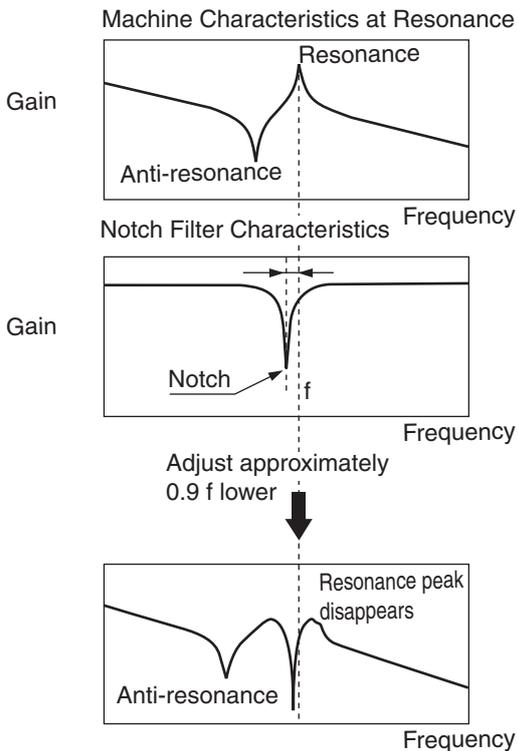
Torque Command Filter Function
