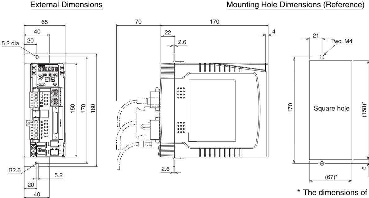
Dimensions for front panel mounting are reference values that provide leeway.
