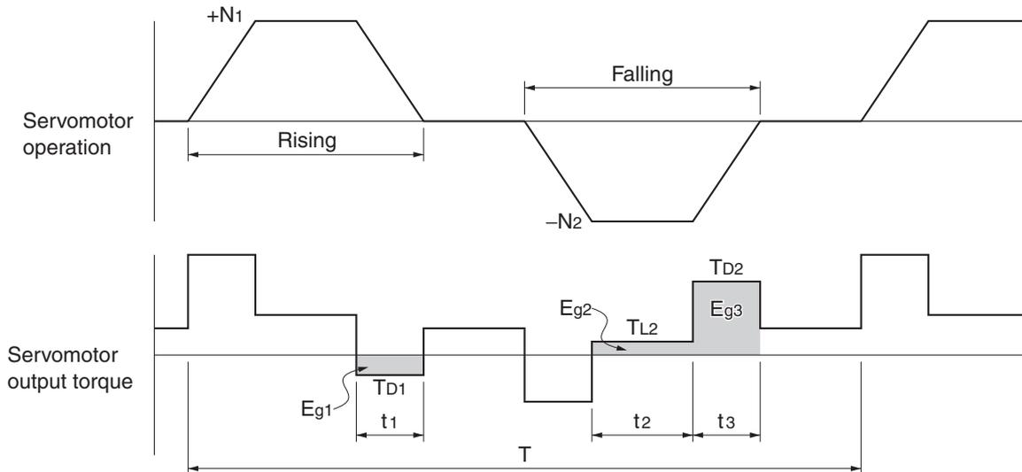
**Note** In the output torque graph, acceleration in the positive direction (rising) is shown as positive, and acceleration in the negative direction (falling) is shown as negative.
