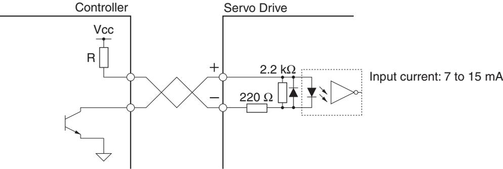
**Note** Select a value for resistance R so that the input current will be from 7 to 15 mA. Refer to the following table.
