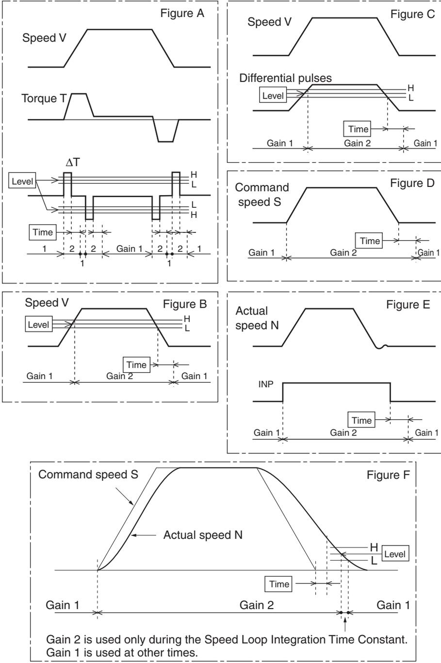
Gain 2 is used only during the Speed Loop Integration Time Constant. Gain 1 is used at other times.
