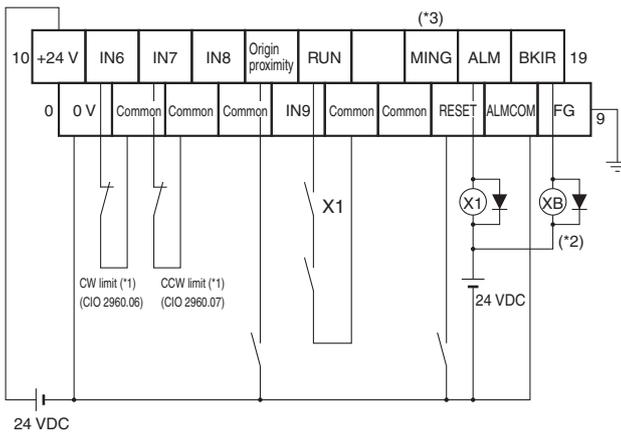
\*1. CW and CCW limit input signals can also be input through Input Units.
