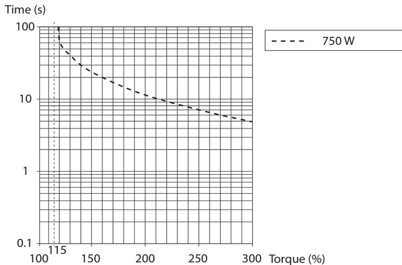
When the torque command = 0, and a constant torque command is continuously applied after three or more times the overload time constant has elapsed, the overload time  $t$  [s] will be:
