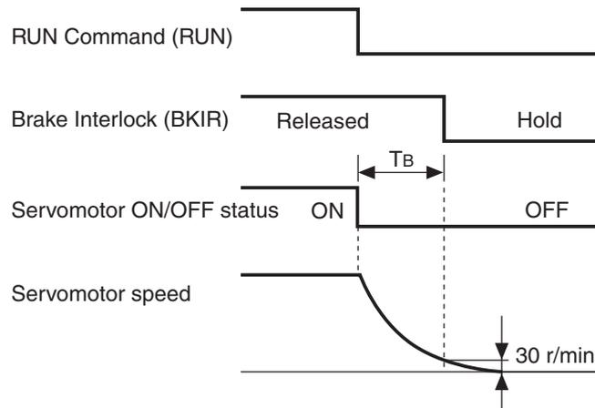
“TB” in the above figure is the brake timing during operation (setting × 2 ms) or the time until the speed of the Servomotor falls to 30 r/min or lower, whichever is shorter.
