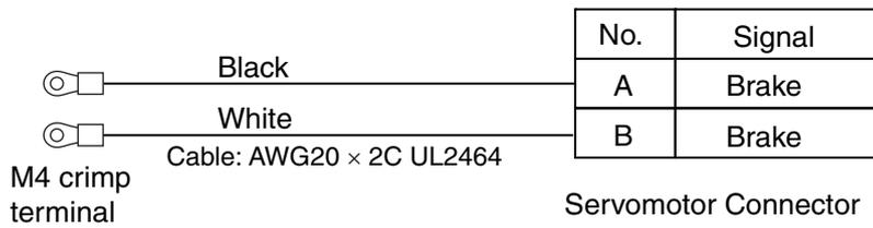
■ European Cables for Brakes (Flexible Cables)
