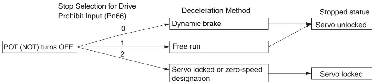
While the Forward Drive Prohibit Input (POT) is OFF, the Servomotor cannot be driven in the forward direction, but it can be driven in the reverse direction. Conversely, while the Reverse Drive Prohibit Input (NOT) is OFF, the Servomotor cannot be driven in the reverse direction, but it can be driven in the forward direction.
