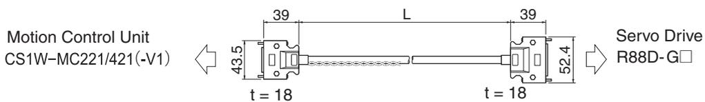
• Cables for Two Axes
