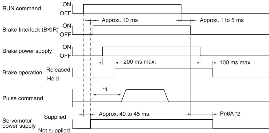
\*1. The time from turning ON the brake power supply to releasing the brake is 200 ms max. Provide a pulse command after the brake has been released, taking into account this delay.
