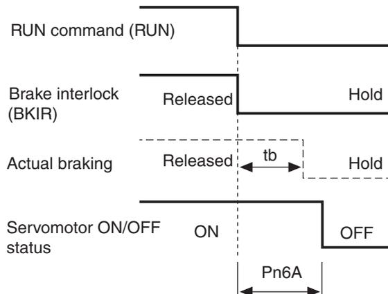
♦ Make the setting as follows to prevent the machine (workpiece) from moving or falling due to the delay in the brake operation (tb).
