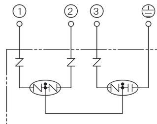
■ Noise Filter for the Power Supply Input
