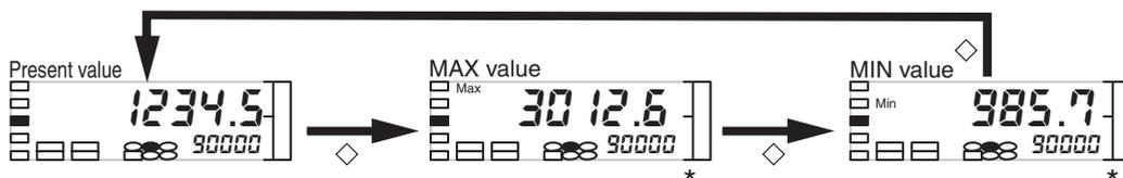
\* If input error enable (*5.Err*) is ON and a sensor error occurs, the input error will be displayed on the maximum and minimum display.
