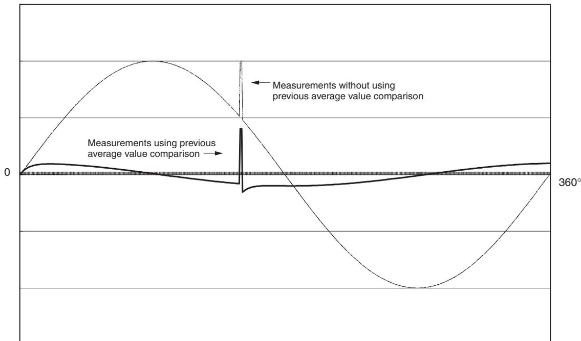
Previous average value comparison makes the measurement value the difference between the present input value and the average of all previous input values.
