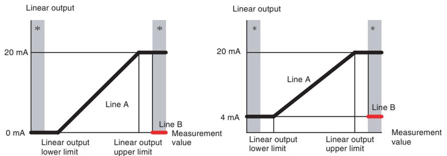
\* Areas marked with an asterisk (\*) are input error areas. If the “operation at input error” parameter is set to “input error,” then the output would be like Line B. Otherwise, the output would be like Line A.
