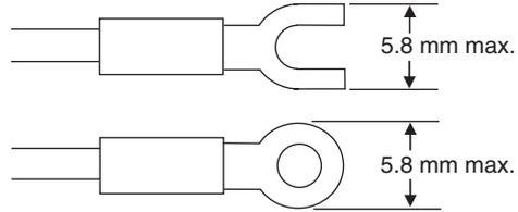
Use cables with a heat resistance of at least 70°C.
