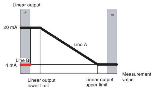
\* If the upper and lower limit are set to the same value, then the upper limit will equals the lower limit plus 1 for linear output.
