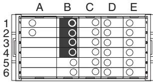
Linear currents and voltages are output between terminals B1 to B2 and between B3 to B4.
