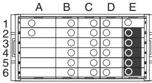
Input the signal to be measured. The following figure shows the inputs that can be measured by each model. Connect the input devices to the terminals shown below according to the input type.
