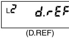
When measurement values change rapidly and the display changes with the measurement values, flickering often occurs and the display becomes difficult to read. The flickering can be suppressed and the display made easier to read in such situations by delaying the display refresh period. The display refresh period is set using the following parameter.
