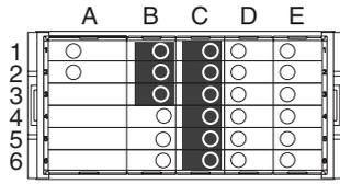
Comparative outputs are output to terminals B1 to B3 and C1 to C6.
