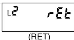
If no keys are operated for a specified time after switching the display in the RUN level or adjustment level, the display will automatically return to the RUN level. The time until the display returns automatically can be set and the automatic display return can be disabled through this setting.
