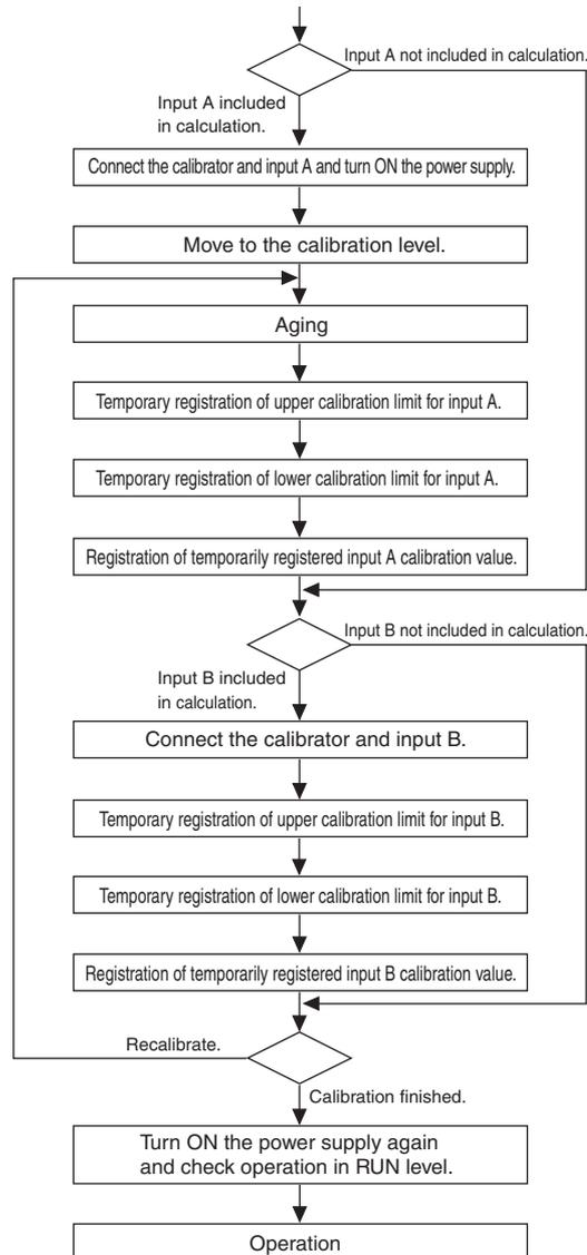
The input type that can be calibrated according to this flowchart is the type selected under “input type A” or “input type B.” To calibrate other input types, switch the setting for “input type A” or “input type B” in the initial setting level to the desired input type and then perform calibration according to the flowchart outlined above.
