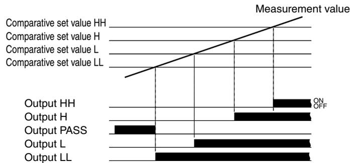
\* The PASS output turns ON when any of the HH, H, L, or LL output turns OFF.
