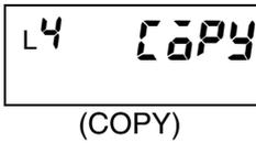
The bank copy function is used to specify a bank between 0 and 7 and copy the group of comparative set values in that bank to all banks.
