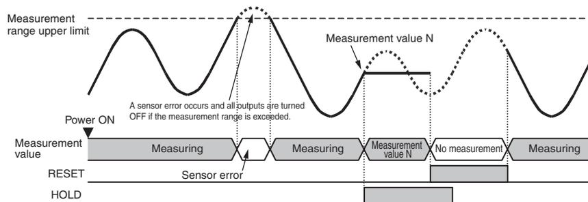
The PV display will show "-----" during RESET input (no measurement status).
