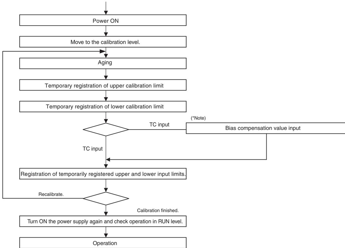
\* The previous calibration value is not displayed when the status of bias compensation values is being monitored. The display cannot handle bias compensation values because they are temperature readings rather than a count. This means the value that is read during calibration is not a bias value, but the calibration value for the main input.
