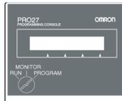
In this example, the Programming Console is used to set the Watch Cycle Time (maximum cycle time) in 10-ms units.
